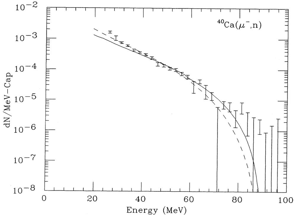
FIG. 3. The histogram shows the neutron spectrum for the reaction  $^{40}\text{Ca}(\mu^-, n)$  (Ref. 1). The solid and dashed curves are ALICE fits to the spectrum with weighted cascades from an  $nh$  and  $nnh$  configuration, respectively. See corresponding proton curves in Fig. 2 and also text.
