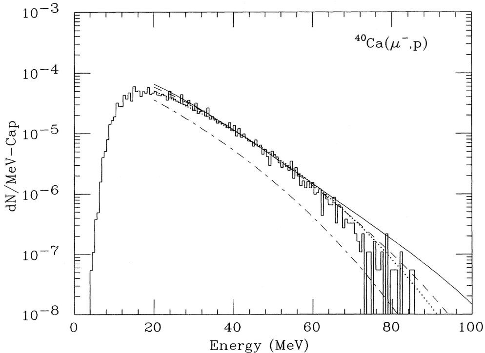
FIG. 2. The histogram shows the measured proton energy spectrum (without corrections) for the reaction  $^{40}\text{Ca}(\mu^-, p)$ . The solid and dashed curves represent phenomenological fits explained in the text. The long-short dashed curve is the proton result when the neutron spectrum (Fig. 3) is fitted with weighted cascades from an *nh* configuration. The dotted curve results when an *nnh* configuration is used. See text.
