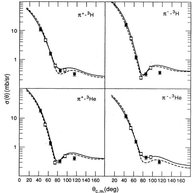
FIG. 1. Angular distributions for the four nuclei considered. The agreement with the data is moderate. The solid curves correspond to case “ $I$ ” and the dotted to case “ $A$ .” While there is not much to distinguish the two to the eye, the case “ $I$ ” gives a much better representation of  $\rho^+$  and  $\rho^-$  at  $45^\circ$ .
