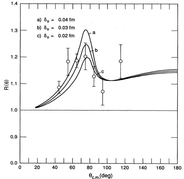
FIG. 2. Example variations with respect to the odd-neutron radius of the calculated “ $R$ ” compared with the data. It is clear that the minimum region (where the “spin-flip” term, depending only on the odd-nucleon form factor, dominates) controls the fit to the data. The curves are calculated for  $r_e^n$  fixed at  $1.720$  fm and  $r_o^n$  taking values of  $1.58$ ,  $1.59$ , and  $1.60$  fm for case “ $A$ .”
