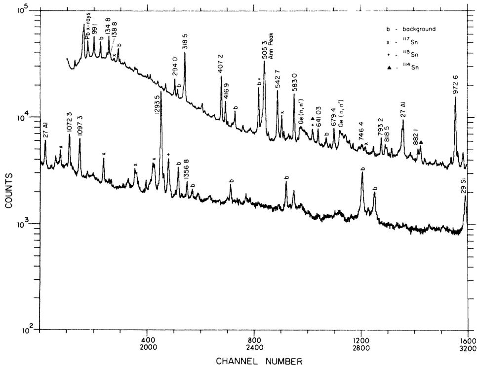
FIG. 2. Typical  $\gamma$ -ray singles spectrum obtained from bombardment of enriched  $^{116}\text{Sn}$  with 50 MeV alpha particles, taken with a 25% HPGe detector placed at  $90^\circ$  to the incident beam direction.
