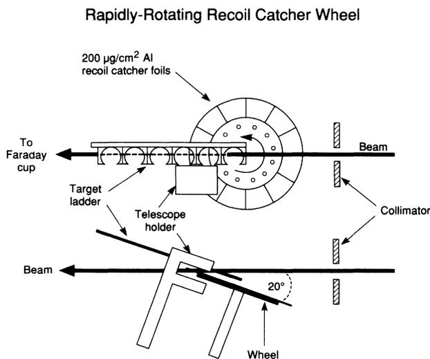
FIG. 2. A schematic diagram of the rapidly rotating recoil-catcher wheel used to search for the g.s. proton decay of <sup>65</sup>As and <sup>69</sup>Br (see text).
