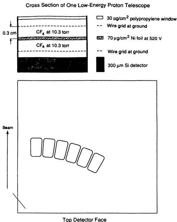
FIG. 3. A cross section of a single low-energy particle-identification telescope and the top view of one telescope array used to search for the g.s. proton decay of  $^{65}\text{As}$  and  $^{69}\text{Br}$ .
