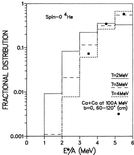
FIG. 5. Fractional distribution of excitation energies per nucleon predicted for the computational zero spin  ${}^4\text{He}$  nuclei (subject to cluster constraint) for temperatures of 2, 3, and 4 MeV (histograms). The points are from the simulated Ca+Ca reaction at  $100A$  MeV and  $b=0$  fm. All distributions have been normalized to unity over the  $0A-6.0A$  MeV range in excitation energy. The  ${}^4\text{He}$  nuclei were observed in the  $60-120$  deg range in the c.m. frame.
