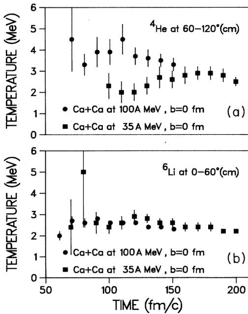
FIG. 9. Comparison of the chemical temperatures obtained in the Ca + Ca reaction at 35 A MeV and 100 A MeV bombarding energy. The top part (a) of the figure is for  ${}^4\text{He}$  nuclei in the angular range of 60–120 deg, while the lower part (b) is for  ${}^6\text{Li}$  in the angular range of 0–60 deg.
