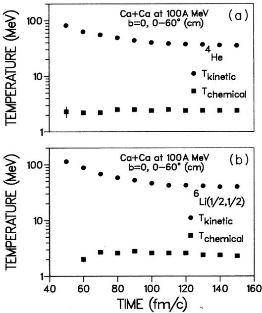
FIG. 8. Time dependence of the kinetic and chemical temperatures for nuclei emitted at 0–60 deg in the Ca + Ca reaction at 100 A MeV. The upper part of the figure (a) is for  ${}^4\text{He}$  nuclei while the lower part (b) is for  ${}^6\text{Li}(\frac{1}{2}, \frac{1}{2})$ .
