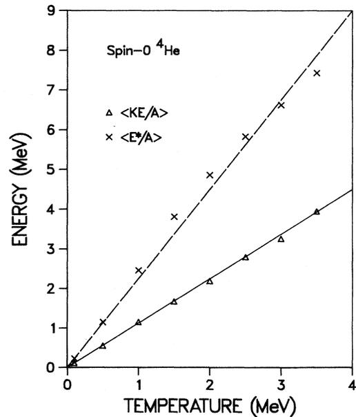
FIG. 1. Calculated kinetic energy per nucleon and excitation energy per nucleon as a function of temperature for computational zero spin  ${}^4\text{He}$  nuclei.
