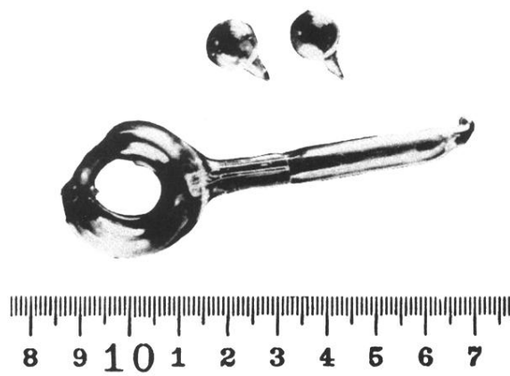
FIG. 4. Photograph of optical-pumping cell, and of spherical electrodeless lamps.
