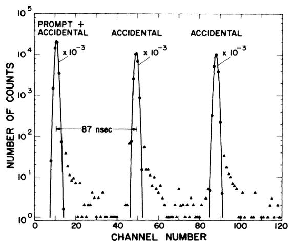
FIG. 2. Typical time spectrum for proton-fission coincidence events from the  $^{235}\text{U}(d,p)$  reaction.
