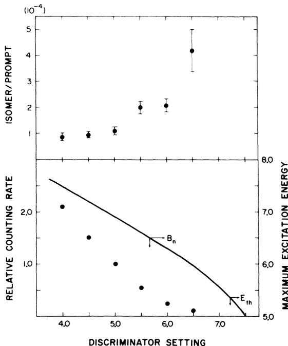
FIG. 4. Bottom half shows the relative proton counting rate as a function of the fast-discriminator setting (points) and a conversion between proton fast-discriminator setting and the maximum excitation energy in  $^{236}\text{U}$  (solid line). Top half shows the measured ratio of isomeric prompt-fission events from the  $(d,p)$  reaction as a function of the proton fast-discriminator setting.
