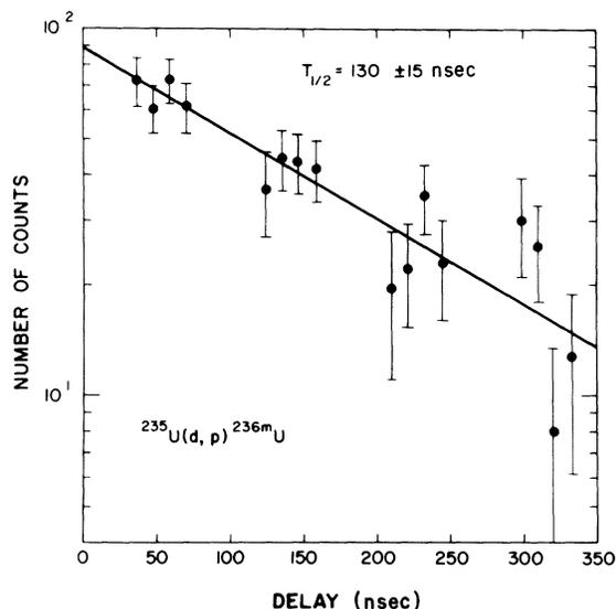
FIG. 3. Time spectrum for delayed events. Results are the sum of all runs and have been corrected for accidental contributions as described in the text. The solid line is a least-squares-fitted function with the indicated half-life.
