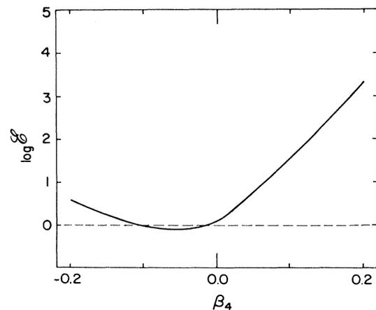
FIG. 3. Enhancement  $\mathcal{E}$  as a function of  $\beta_4$  for the reaction  $^{16}\text{O} + ^{232}\text{Th}$ . A value of  $\beta_2=0.2$  was used, somewhat smaller to the prolate deformation assumed in Ref. 2. The enhancements are normalized to the value obtained for  $\beta_4=0$  and thus reflect directly the role of the hexadecapole degree of freedom in this particular case.
