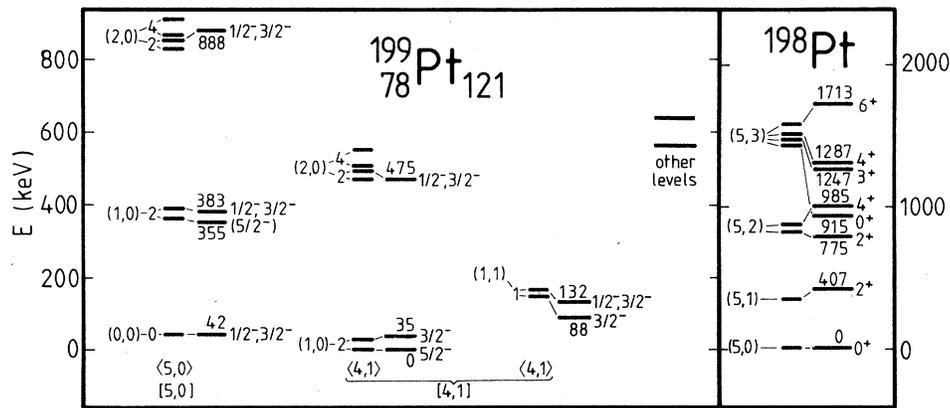
FIG. 4. Same as Fig. 2, but for the isotopes  $^{199}\text{Pt}$  and  $^{198}\text{Pt}$  ( $n_b + n_f = 5$ ).
