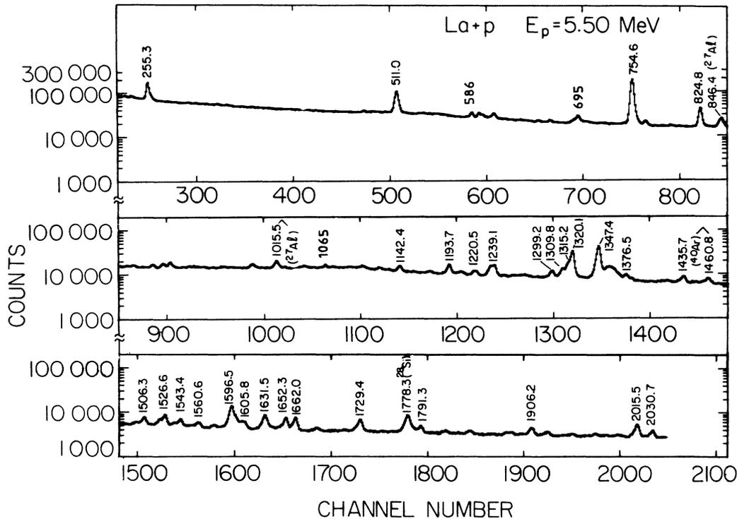
FIG. 1. Gamma-ray spectrum observed with a 50 cm<sup>3</sup> Ge(Li) detector following the bombardment of a lanthanum target with 5.50 MeV protons.
