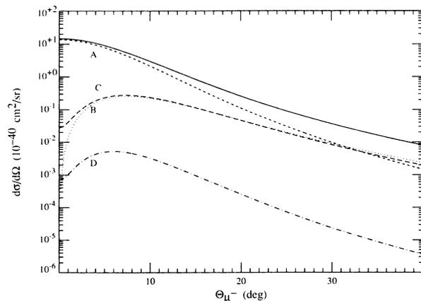
FIG. 3. Plot of the differential cross section for the reaction  $\nu_\mu + {}^{12}\text{C} \rightarrow {}^{12}\text{N} + \mu^-$  as a function of outgoing muon laboratory angle for 1 GeV neutrinos. Curves A, B, C, and D refer to the contribution from  $F_A$ ,  $F_M$ ,  $F_E$ , and  $F_P$ , respectively.
