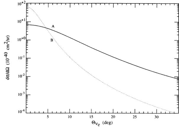
FIG. 2. Plot of the differential cross section for the reaction  $e^- + {}^{12}\text{C} \rightarrow {}^{12}\text{B} + \nu_e$  as a function of outgoing muon laboratory angle. Curves A and B are for 1 GeV and 3 GeV incident electrons, respectively.
