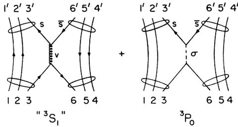
FIG. 1. Lowest order diagrams for  $p\bar{p} \rightarrow \Lambda\bar{\Lambda}$ . The scalar exchange is called  $\sigma$  in analogy to the topological soliton model (Ref. 12).
