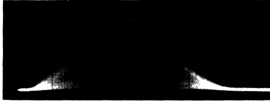
FIG. 6. Output signals of the trapezoidal DL-RC shaper. X scale, 400 ns/div; Y scale, 0.5 V/div. A ^{60}\text{Co} source was used.
