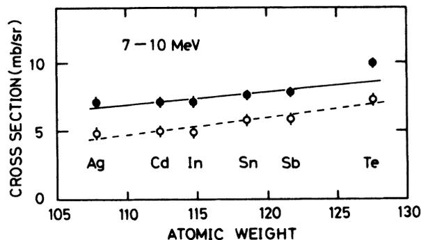
FIG. 3. Dependence of integrated cross sections over 7–10 MeV on the atomic weight of scatterers. Solid circles represent the measured cross sections at  $70^\circ$ . Open circles are the results after subtraction of the predicted LEOR cross sections. Error bars represent only the statistical errors.
