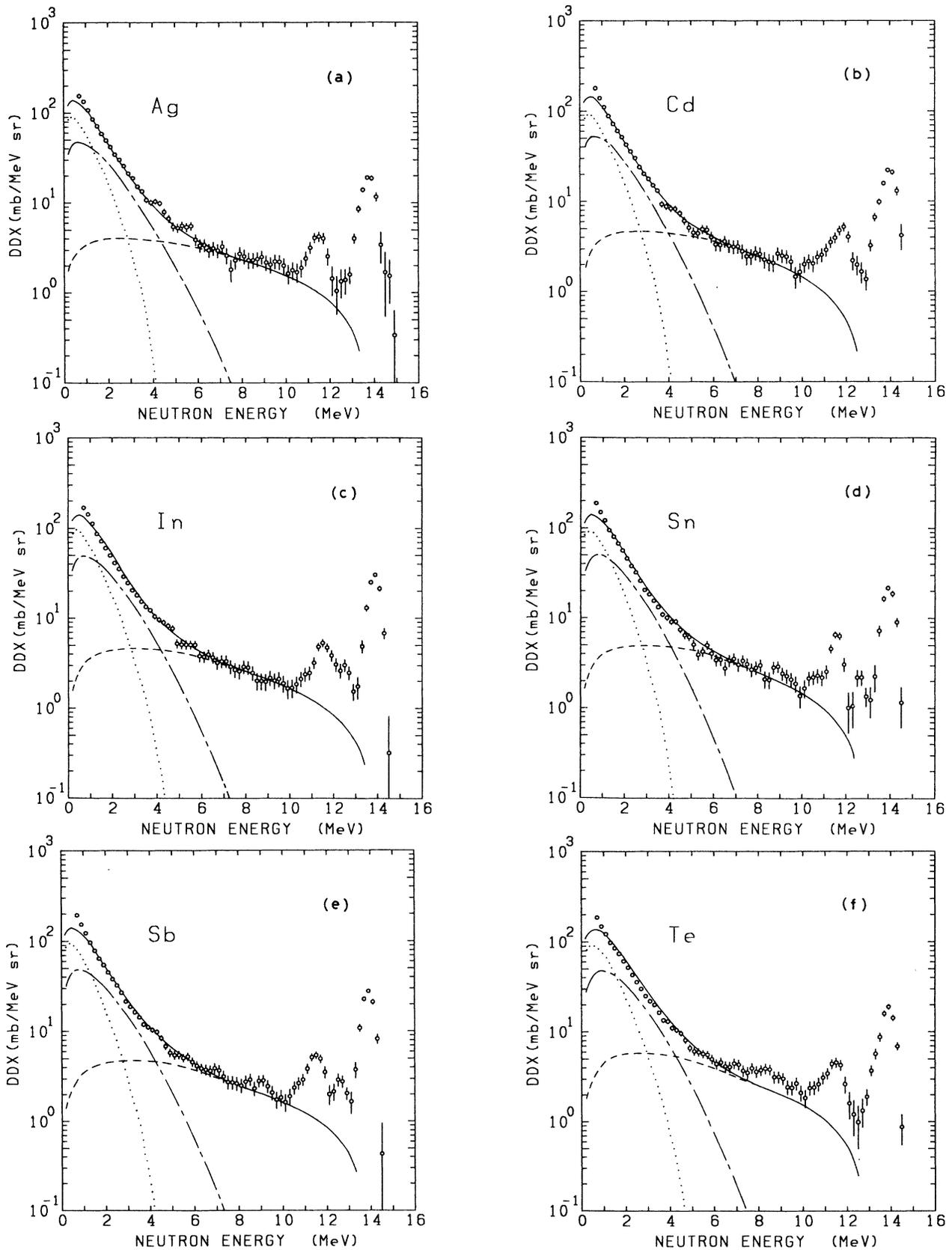
FIG. 2. Comparisons of the experimental and calculated double differential neutron emission cross sections for Ag, Cd, In, Sn, Sb, and Te at  $70^\circ$ . Dashed curves are the calculated preequilibrium spectra using the exciton model. Dot-dashed curves and dotted curves show the calculated evaporation spectra for emissions of one neutron and two neutrons, respectively. Solid curves are the sum of them.
