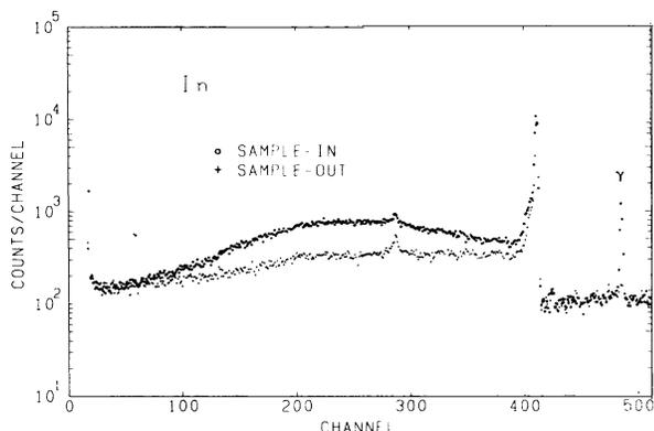
FIG. 1. Time-of-flight spectrum of  $70^\circ$  for the  $\text{In}(n,xn)$  reaction at 14.1 MeV and the associated background spectrum.
