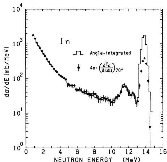
FIG. 4. Comparison of the angle-integrated energy spectrum (histogram) and  $4\pi$  times the energy spectrum at  $70^\circ$  (solid circles) measured for the  $\text{In}(n,xn)$  reaction.
