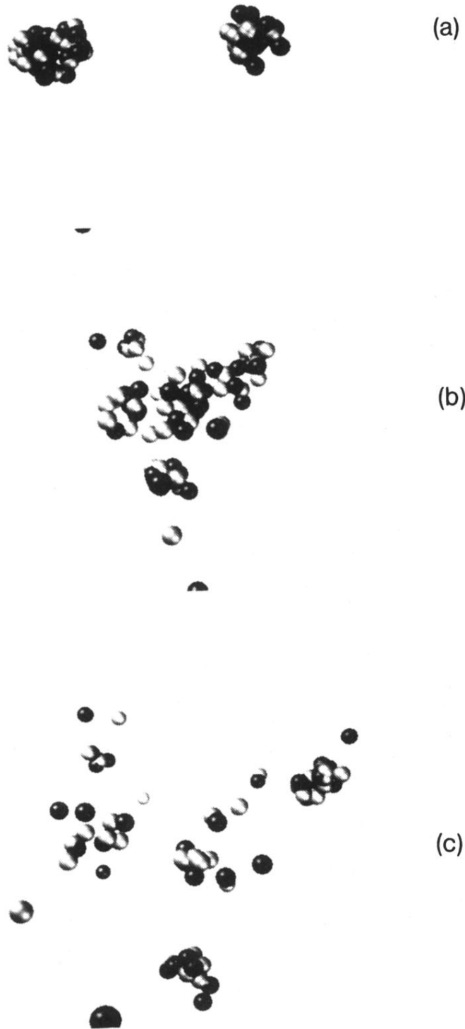
FIG. 3. Time evolution of a central Ca + Ca collision at 50 MeV/nucleon bombarding energy. Same representation as Fig. 1.
