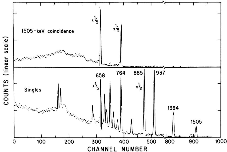
FIG. 8. Singles (bottom) and 1505-keV coincidence spectra of  $^{110}\text{Ag}^m$  decay. The small peaks in the coincidence spectrum are from accidental coincidences.
