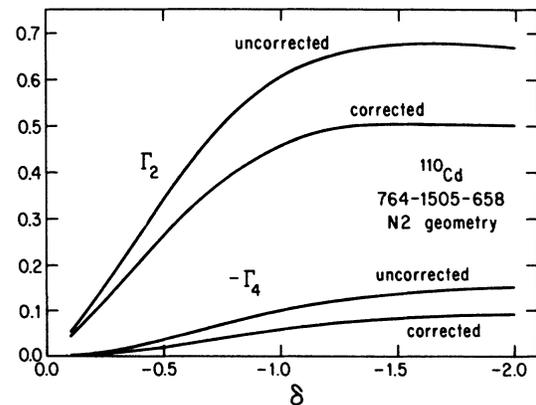
FIG. 5. Triple angular distribution coefficients  $\Gamma_2$  and  $\Gamma_4$  for the 764-1505-658 keV cascade in  $^{110}\text{Cd}$  in the  $N2$  geometry. Note that the negative of  $\Gamma_4$  is plotted.
