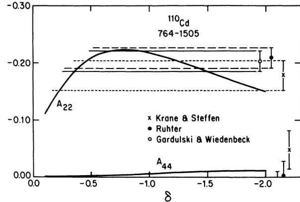
FIG. 2. Angular correlation coefficients  $A_{22}$  and  $A_{44}$  vs  $\delta$  for the 764-1505 keV cascade in  $^{110}\text{Cd}$ .
