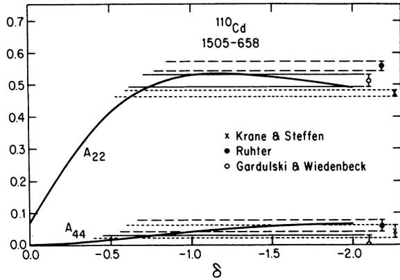
FIG. 3. Angular correlation coefficients  $A_{22}$  and  $A_{44}$  vs  $\delta$  for the 1505-658 keV cascade in  $^{110}\text{Cd}$ .
