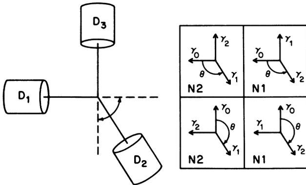
FIG. 6. Geometry of the triple correlation experiment. The three detectors lie in a plane with  $D_1$  (Ge) and  $D_3$  (NaI) at  $90^\circ$  to one another and  $D_2$  (Ge) moving in the quadrant shown. By accepting different gammas in the energy windows, the four configurations shown at right can be achieved.
