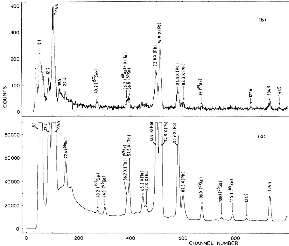
FIG. 3. Partial low energy  $\gamma$  spectrum recorded with the intrinsic Ge photon spectrometer. (a) Direct spectrum; (b) gated by a liquid scintillator neutron counter ( $0^\circ$  to beam). The energies of the  $\gamma$ -ray peaks are given in keV. The transitions without labels are either unidentified or known contaminants.
