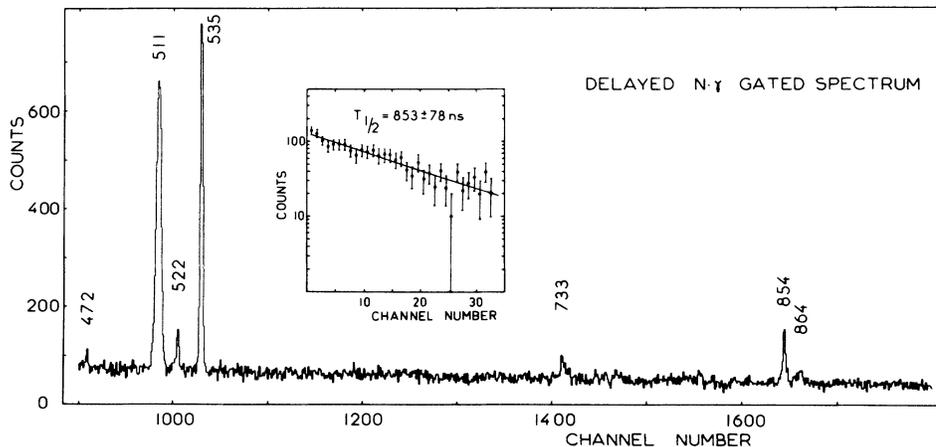
FIG. 4. Portion of a 4096-channel spectrum in delayed coincidences gated with neutrons and with  $\gamma$  rays between 0.1 and 3.0 MeV. The time window begins 130 ns after the prompt peak and is open during  $2 \mu\text{s}$ . In the inset, the decay curve of the 535 keV  $\gamma$  ray is reported, with the background subtracted. In that case, each channel corresponds to 60 ns.
