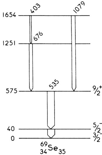
FIG. 6. Level scheme for  $^{69}\text{Se}$  including the first excited states populated in the  $^{40}\text{Ca}(^{32}\text{S},2\text{pn})^{69}\text{Se}$  reaction. The  $\gamma$  intensities are roughly proportional to the width of the arrows.
