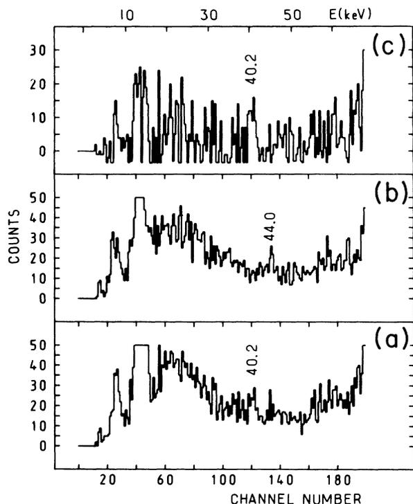
FIG. 5. Portion of  $\gamma$ - $\gamma$  coincidence spectrum recorded at  $E(^{32}\text{S})=103$  MeV, gated by (a) the 535 keV transition in  $^{69}\text{Se}$ , (b) the corresponding background, and (c) the 535 keV line after background subtraction. The  $^{66}\text{Ga}$  transition of 44 keV observed on backgrounds is due to the  $^{66}\text{Ge}$  beta decay. The 40 keV assignment ( $^{60}\text{Se}$ ) is discussed in the text.
