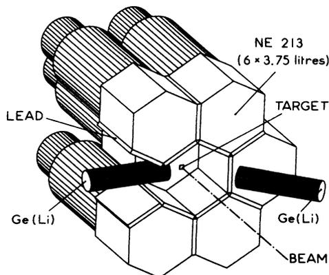
FIG. 1. Schematic diagram of the experimental setup.
