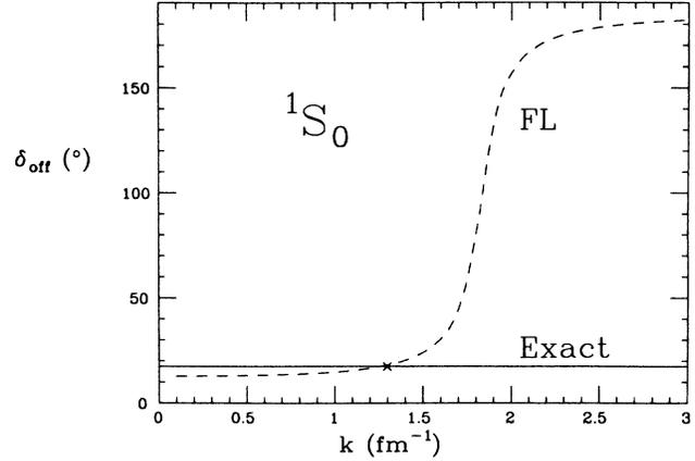
FIG. 4. Half-shell phase shift  $\delta_l(k,p)$  for the FL  $^1S_0$  state at 140 MeV (dashed line). If the half-shell amplitude satisfied unitarity it would be constant (solid line). The on-shell point is marked by an  $\times$ .
