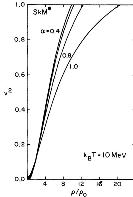
FIG. 1. Dependence of the speed of sound in nuclear matter on the asymmetric coefficient  $\alpha$ , for interaction SkM\* and temperature  $k_B T = 10$  MeV.  $\rho_0$  is the normal nuclear matter density ( $0.16 \text{ fm}^{-3}$ ).
