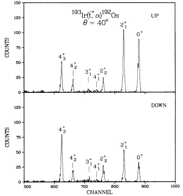
FIG. 2. Portion of the spectrum of the  $^{193}\text{Ir}(t, \alpha)^{192}\text{Os}$  reaction at  $40^\circ$  with spin "up" and "down." States are labeled by their known (Ref. 17)  $J^\pi$  values.
