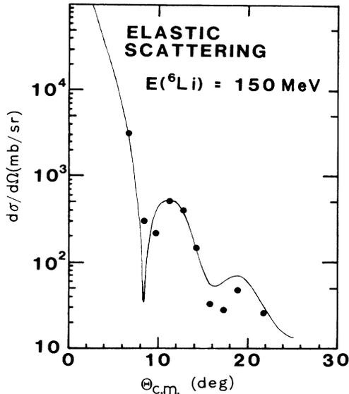
FIG. 2. Observed and calculated angular distributions of elastic scattering for  ${}^6\text{Li} + {}^{12}\text{C}$  at  $E_{\text{lab}} = 150$  MeV.
