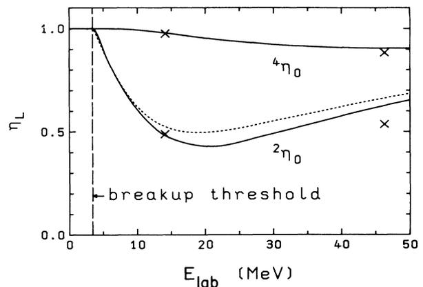
FIG. 6. Doublet and quartet  $S$ -wave inelasticities, crosses are from Ref. 3. The solid-line doublet inelasticity results from the optimized choice  $k = k_t = 0.655 \text{ fm}^{-1}$ , whereas the dashed line corresponds to  $k=0$  (see text).
