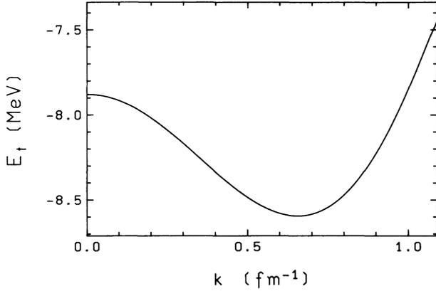
FIG. 2. Variation of the triton binding energy  $E_t$  with the negative-energy  $W$ -matrix parameter  $k$  [cf. Eqs. (5) and (6)].
