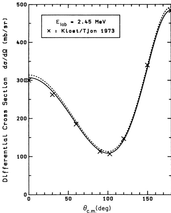
FIG. 7. Differential cross section at  $E_{\text{lab}} = 2.45$  MeV; crosses are from Ref. 3 (see text). The solid line corresponds to the optimized choice  $k = k_i = 0.655$  fm $^{-1}$ , whereas the dashed line corresponds to  $k = 0$  (see text).
