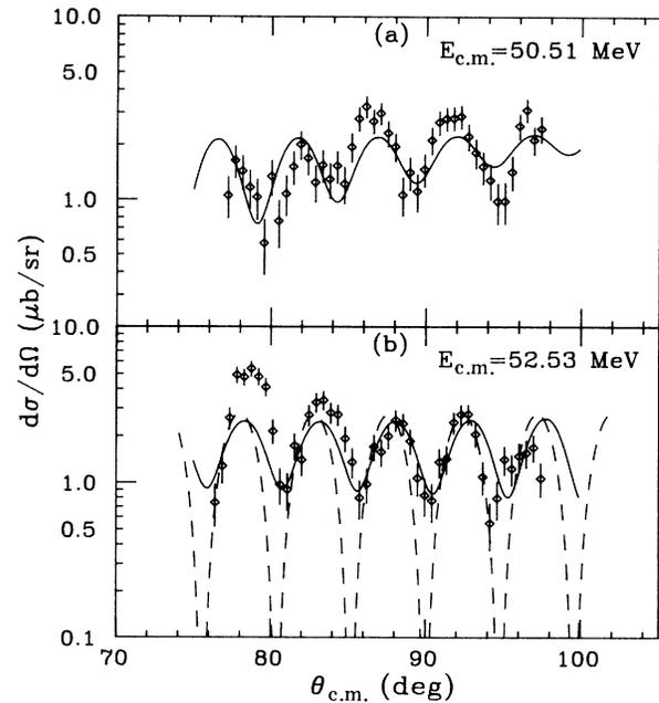
FIG. 5. Elastic scattering angular distributions measured at (a)  $E_{c.m.}=50.51$  MeV and (b)  $E_{c.m.}=52.53$  MeV. The solid curve in (a) is a fit involving  $l=33$ ,  $34$ , and  $35$  with amplitudes of  $0.65$ ,  $0.70$ , and  $0.60$ , respectively. The solid curve in (b) is a fit with  $l=36$ ,  $37$ , and  $38$  with amplitudes of  $0.10$ ,  $1.00$ , and  $0.60$ , respectively. The dashed curve in (b) is  $P_{37}^2(\cos\theta_{c.m.})$ .
