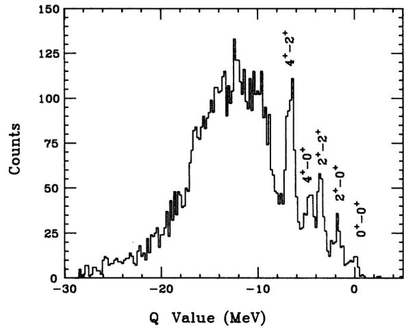
FIG. 2.  $Q$ -value spectrum measured at a bombarding energy of  $E_{\text{lab}}=97.40$  MeV. The peak labeled  $2^+-0^+$  contains contributions from both the  $^{24}\text{Mg}$   $2^+$  (1.37 MeV) and the  $^{28}\text{Si}$   $2^+$  (1.78 MeV) states. The peak labeled  $4^+-0^+$  contains contributions from the  $^{24}\text{Mg}$   $4^+$  (4.12 MeV) and the  $^{28}\text{Si}$   $4^+$  (4.62 MeV) states. The peak labeled  $4^+-2^+$  contains contributions from both  $2^+$  and  $4^+$  excitations.
