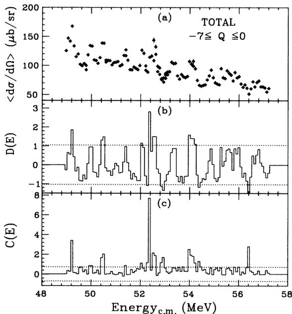
FIG. 4. Results of a statistical fluctuation analysis of the present data similar to that presented in Ref. 9. (a) Total cross section summed from  $E_x=0.0-7.0$  MeV, (b) summed deviation function  $D(E)$ , and (c) cross correlation function  $C(E)$ . The dotted lines correspond to the 99% confidence levels calculated for statistical fluctuations.
