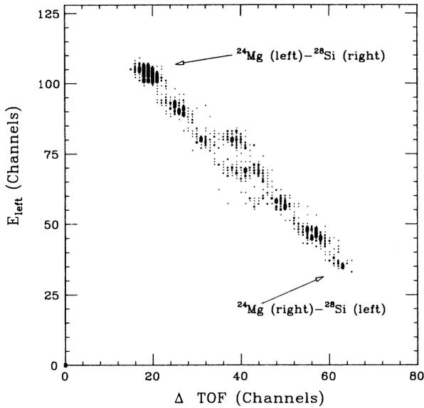
FIG. 1. Particle identification spectrum gated on elastic scattering. The horizontal axis corresponds to the time of flight difference, and the vertical axis the energy of one of the fragments. The two possible detector combinations of the reaction fragments are well separated and the lobes of the elastic scattering angular distribution are clearly visible. The time of flight difference between the two groups is 0.65 ns.
