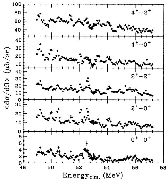
FIG. 3. Excitation functions for elastic and inelastic scattering in  $^{24}\text{Mg}+^{28}\text{Si}$ . The identification of the various channels corresponds to the labeling on Fig. 2.
