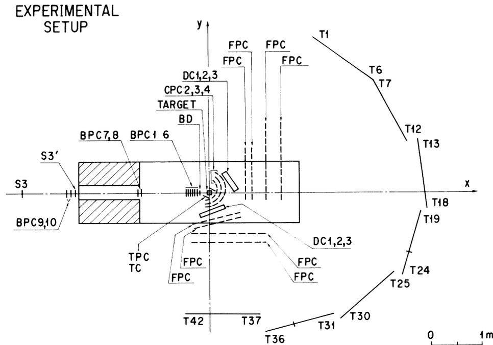
FIG. 1. The layout of counters and chambers inside and outside the spectrometer. (See the text.)
