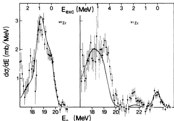
FIG. 5. Comparison of the experimental angle integrated alpha particle spectra at 18.15 MeV incident neutron energy with those calculated by pick-up theory.
