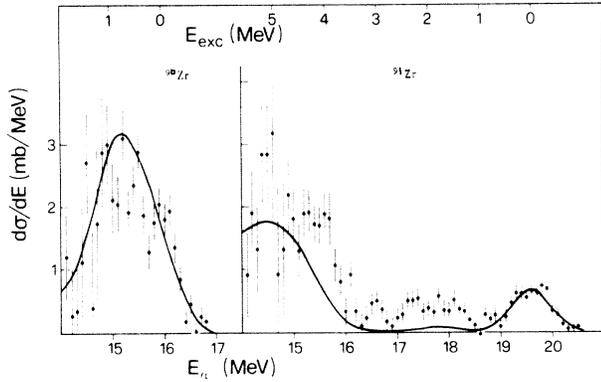
FIG. 2. Comparison of the experimental angle integrated spectra from Zr isotopes at 14.3 MeV incident neutron energy with those calculated by pick-up theory.
