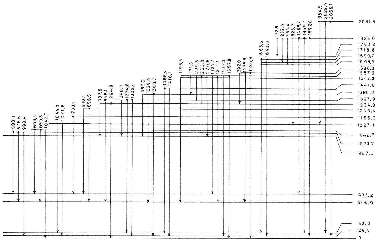
FIG. 2. Partial decay scheme of  $^{105}\text{Ag}$ . Transitions marked with a dot were used to calculate lifetimes.
