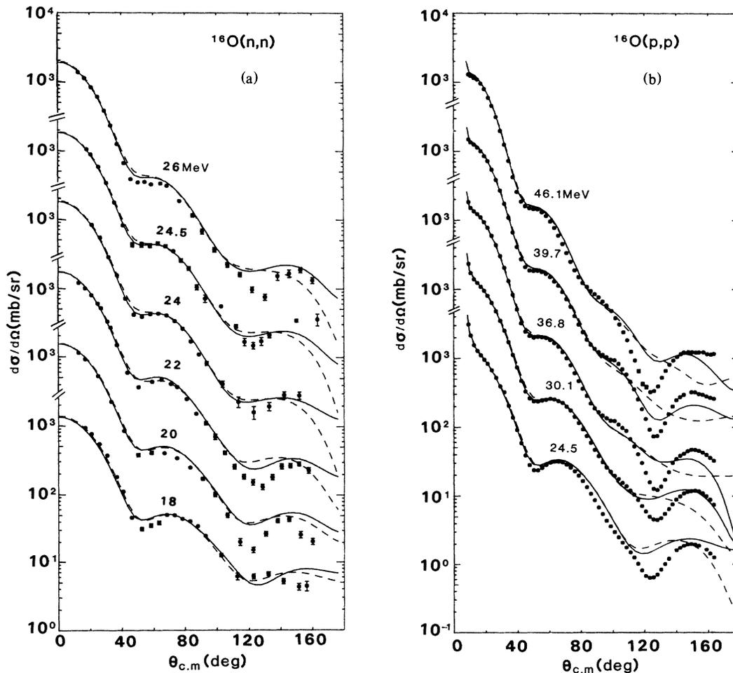
FIG. 1. Elastic scattering of (a) neutrons and (b) protons from  $^{16}\text{O}$ . Solid lines are calculations including coupling to the giant resonance states and to the  $3^-$  state at 6.13 MeV. In all cases  $\beta_3 = 0.56$ . Dashed lines show the effect of excluding the giant resonance couplings.
