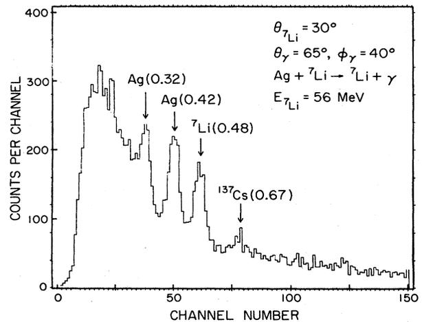
FIG. 3. Laboratory  $\gamma$ -ray spectrum in coincidence with inelastically scattered  $^7\text{Li}$  nuclei at  $50^\circ$ . Production of the low lying silver states near  $0.32$  and  $0.42\text{ MeV}$ , and the lithium state at  $0.48\text{ MeV}$  is clearly shown. The line from the  $^{137}\text{Cs}$  random-calibration source is barely visible.
