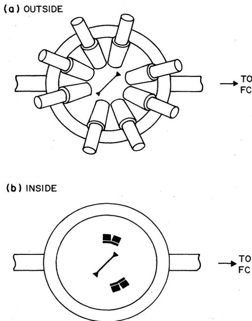
FIG. 2. (a) Schematic diagram of the NaI(Tl) array. The detectors were placed at  $25^\circ$ ,  $65^\circ$ ,  $105^\circ$ ,  $165^\circ$ ,  $205^\circ$ ,  $245^\circ$ ,  $285^\circ$ , and  $345^\circ$  with respect to the beam. (b) Schematic diagram of the particle detectors inside the vacuum chamber.
