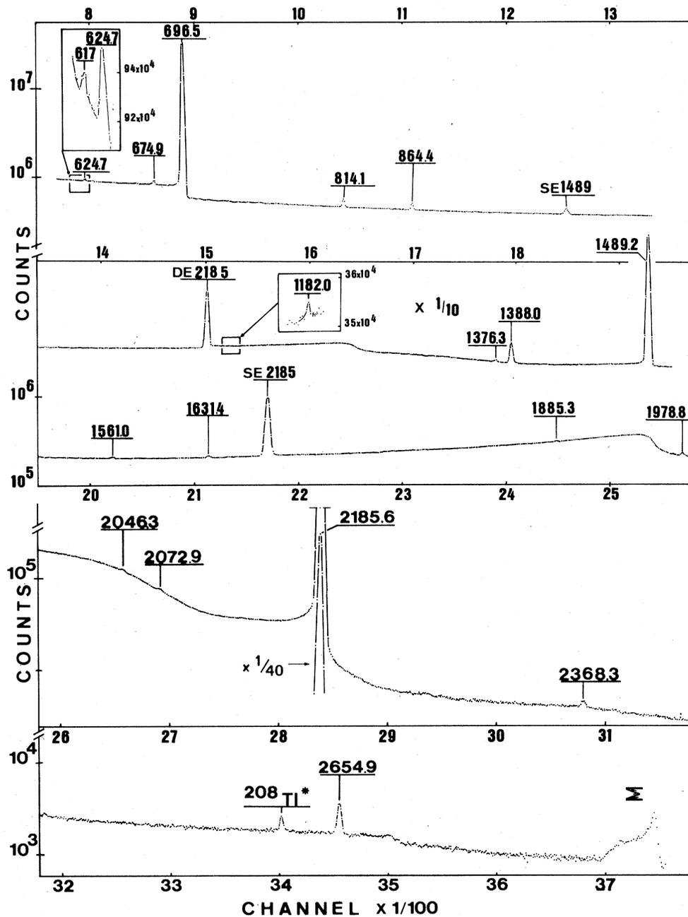
FIG. 1.  $\gamma$ -ray spectrum of  $^{144}\text{Pr}^{m+s}$  isomers in equilibrium with  $^{144}\text{Ce}$ , measured with a 17% HPGe detector. Energies are in keV; the energy dispersion is 0.76 keV/channel. SE and DE stand for single and double escape peaks, respectively. An asterisk denotes a  $\gamma$  ray from the background;  $\Sigma$  indicates summing a peak from 2185.6 and 696.5 keV  $\gamma$  rays.
