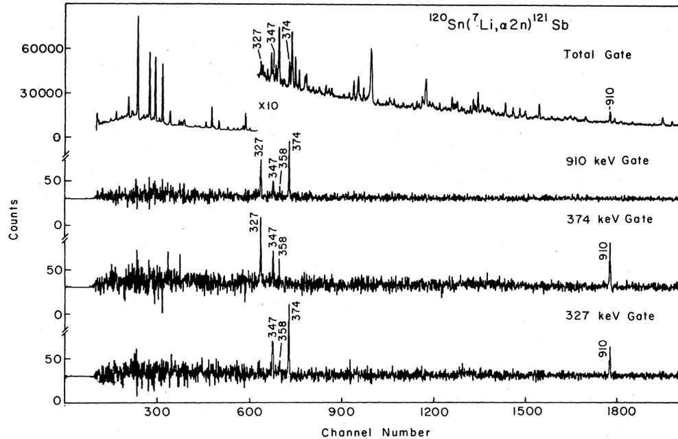
FIG. 5. Background-subtracted  $\gamma$ - $\gamma$  coincidence spectra for the three gates in  $^{121}\text{Sb}$  (bottom). The total  $\gamma$ - $\gamma$  gates spectrum is shown at the top.
