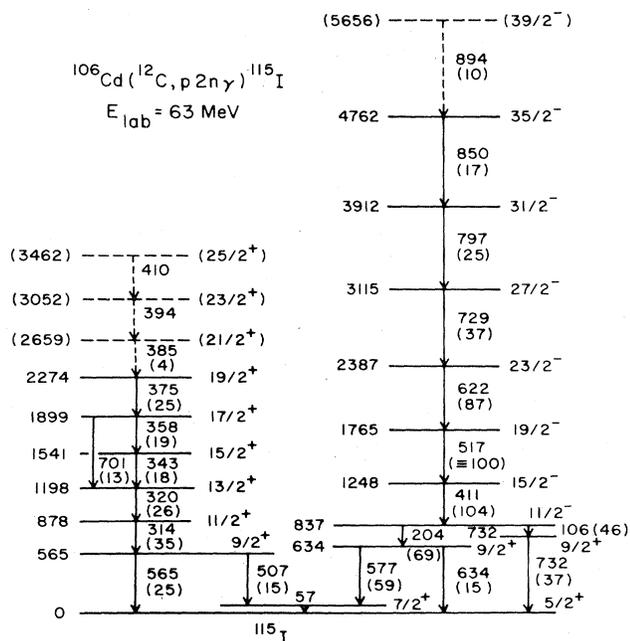
FIG. 2. Level scheme deduced for the  $^{115}\text{I}$  nuclide. All energies are in keV.
