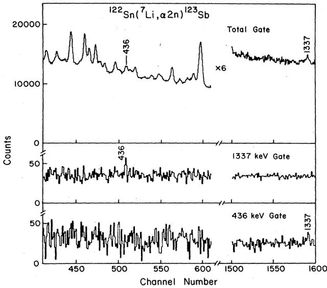
FIG. 7. Background-subtracted  $\gamma$ - $\gamma$  coincidence spectra for two gates in  $^{123}\text{Sb}$  (bottom). The total  $\gamma$ - $\gamma$  gated spectrum is shown at the top.
