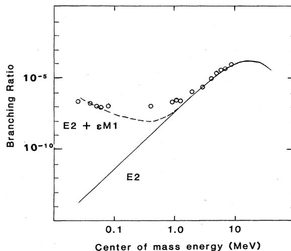
FIG. 5. Comparison of measured branching ratios for the  $^2\text{H}(d,\gamma)^4\text{He}$  reaction to calculated branching ratios. Present measurements are for center of mass energies below 100 keV. The solid curve corresponds to a purely electric quadrupole capture ( $E2$ ) process, while the dashed curve includes an admixture of magnetic dipole capture ( $E2 + \epsilon M1$ ).
