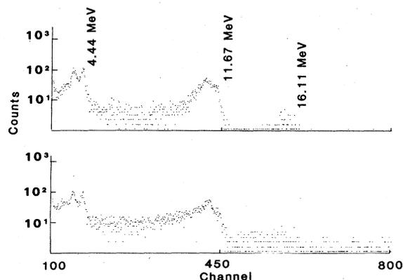
FIG. 2. Gamma ray spectra from the resonant reaction  $^{11}\text{B}(p,\gamma)^{12}\text{C}$  with (top spectrum) and without (bottom spectrum) the annulus anticoincidence condition.
