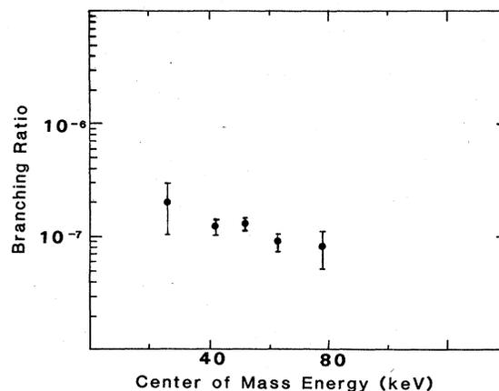
FIG. 4. Measured values of the thick target branching ratios for d-d center of mass energies between 25 and 80 keV.
