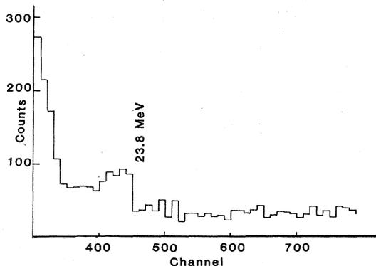
FIG. 3. Gamma ray spectrum from the reaction  $^2\text{H}(d,\gamma)^4\text{He}$  measured at a deuteron bombarding energy of 120 keV. The energy scale in this spectrum is reduced relative to the spectra in Fig. 2.
