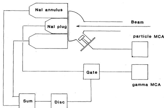
FIG. 1. Schematic layout of experimental setup. The target is located at the back wall of the semicircular scattering chamber and is viewed at  $135^\circ$  deg by the silicon particle detector. The gate on the gamma signal is normally open and is closed by a signal from the annulus.
