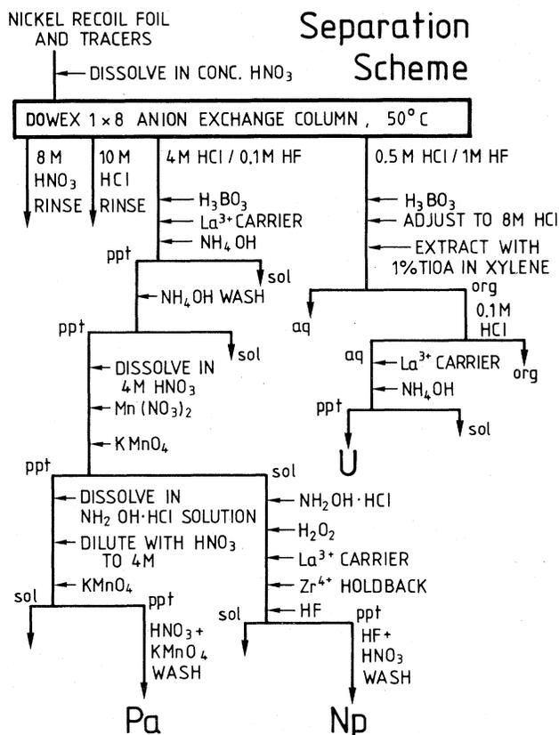
FIG. 1. The chemical separation scheme for preparing samples of protactinium, uranium, and neptunium suitable for use in cross section determinations by means of gamma-ray detection.
