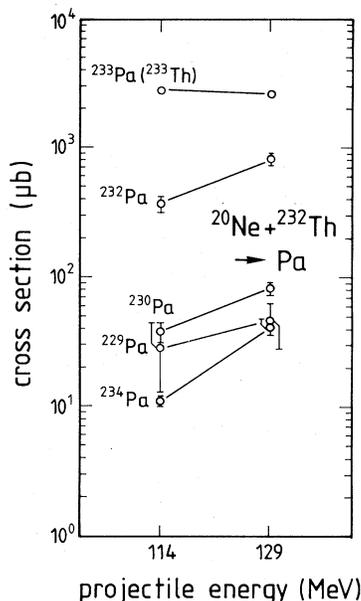
FIG. 5. Partial excitation functions for the protactinium isotopes produced in the bombardment of  $^{232}\text{Th}$  with  $^{20}\text{Ne}$ . Projectile energies are center of target in the laboratory frame.
