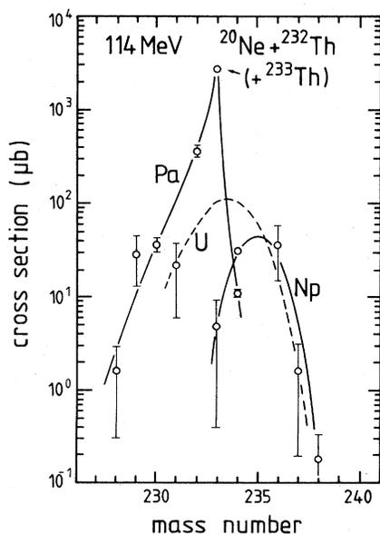
FIG. 3. Product cross sections from the reaction of 114 MeV  $^{20}\text{Ne}$  with  $^{232}\text{Th}$ . Cross sections for nuclides of the same element are connected only to guide the eye.
