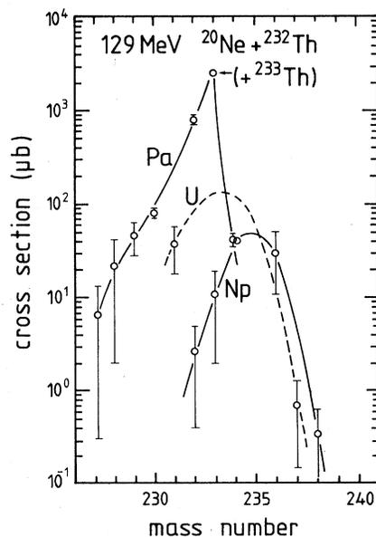
FIG. 4. Product cross sections from the reaction of 129 MeV  $^{20}\text{Ne}$  with  $^{232}\text{Th}$ . Cross sections for nuclides of the same element are connected only to guide the eye.
