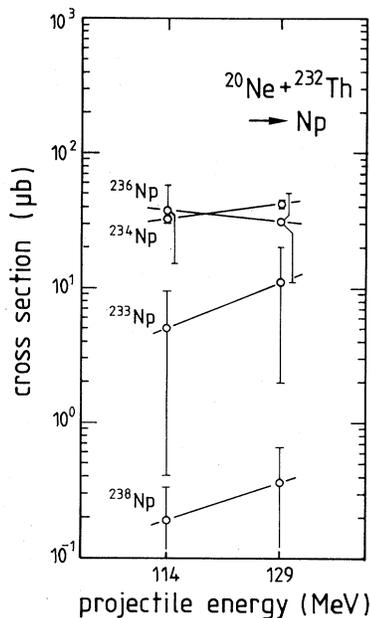
FIG. 6. Partial excitation functions for the neptunium isotopes produced in the bombardment of  $^{232}\text{Th}$  with  $^{20}\text{Ne}$ . Projectile energies are center of target in the laboratory frame.
