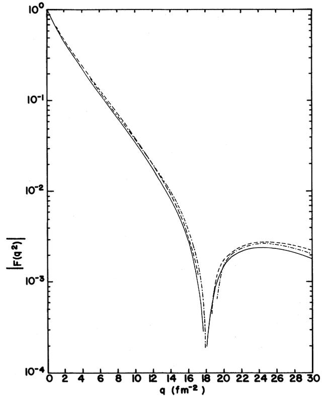
FIG. 3. Charge form factors  $|F(q^2)|$  calculated using the 14-term wave function and Malfliet-Tjon potential  $V$  without three-body force—solid line, with the three-body force  $V_{31}$ —dashed line, with the three-body force  $V_{32}$ —dot dashed line.
