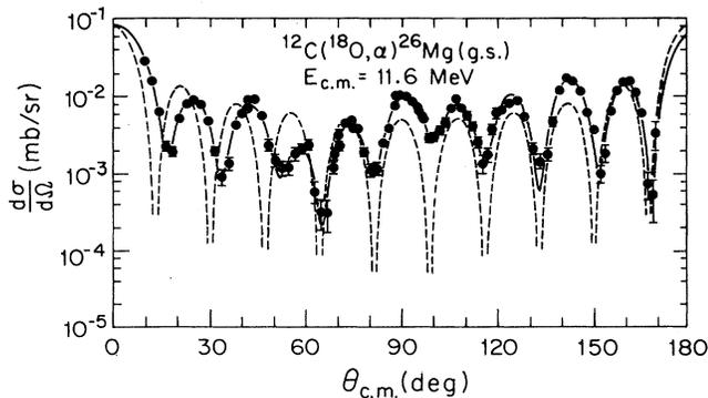
FIG. 3. Angular distribution for  $^{12}\text{C}(^{18}\text{O},\alpha)^{26}\text{Mg}(\text{g.s.})$ , compared with  $P_l$  fit up to  $l=22$  (solid curve) and a pure  $P_{10}^2(\cos\vartheta)$  (dashed curve).
