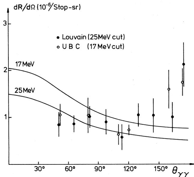
FIG. 1. Angular distribution of the photons in the  $^{12}\text{C}(\pi^-, \gamma\gamma)X$  reaction; full lines are the theoretical predictions of Ref. 5. Energy resolution is included in the theoretical result for 25 MeV photon threshold.
