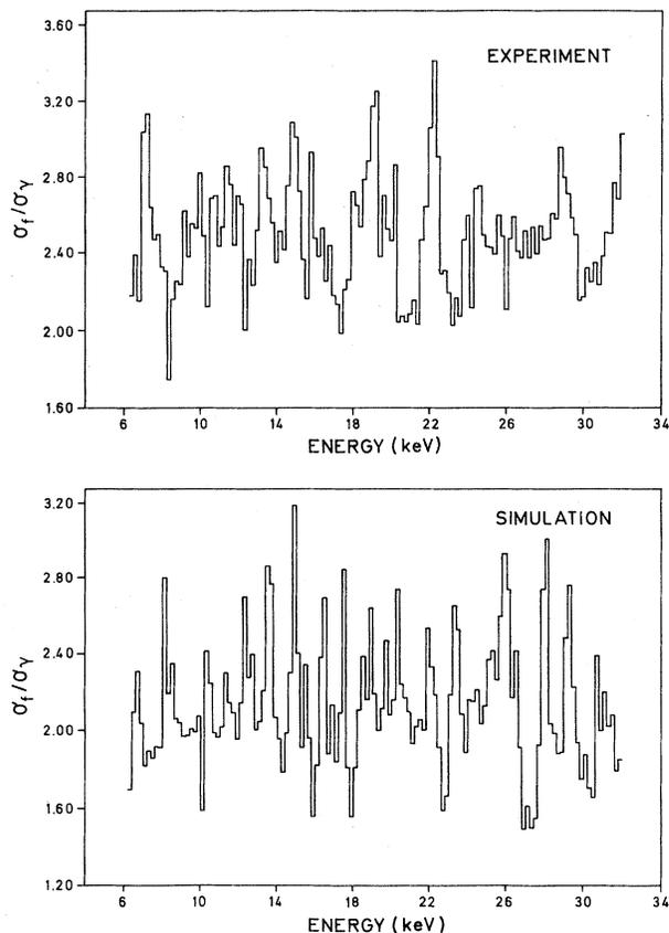
FIG. 2. Comparison of simulated  $\sigma_f/\sigma_\gamma$  for  $D_{II}=280$  eV with the renormalized experimental values; the averaging interval is 200 eV. The experimental data have been multiplied by a smoothly varying energy dependent factor in order to keep the local  $\sigma_f/\sigma_\gamma$  constant over the energy range of interest.
