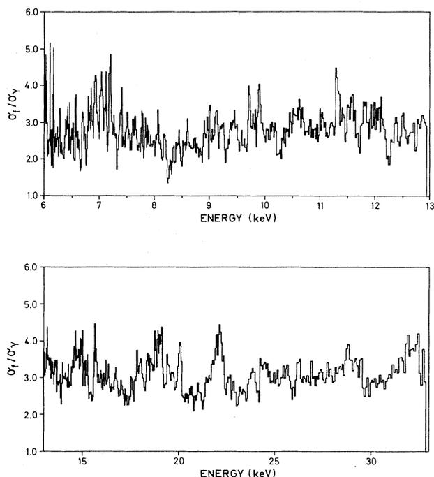
FIG. 1. The fission-to-capture cross-section ratio  $\sigma_f/\sigma_\gamma$  for ( $^{235}\text{U} + n$ ) as measured by Corvi *et al.* (Ref. 12) versus neutron energy from 6 to 32 keV.
