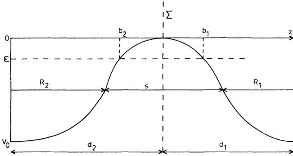
FIG. 2. The nuclear barrier along the  $z$  axis. The distance between the centers of the nuclei is  $d_1 + d_2 = s + R_1 + R_2$ , where  $d_i$  ( $i = 1, 2$ ) is the distance to the surface  $\Sigma$  explained in the text,  $R_i$  the nuclear radii, and  $s$  the distance between surfaces.  $b_i$  are the turning points of the single particle level.
