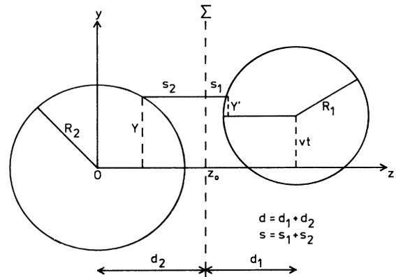
FIG. 1. The geometry of two colliding nuclei. The origin of coordinates is at the center of nucleus 2. Nucleus 1 moves uniformly on a straight line parallel to the  $y$  axis with velocity  $v$ . The distance of closest approach  $d$  is reached at  $t=0$ . The surface  $\Sigma$  is explained in the text.
