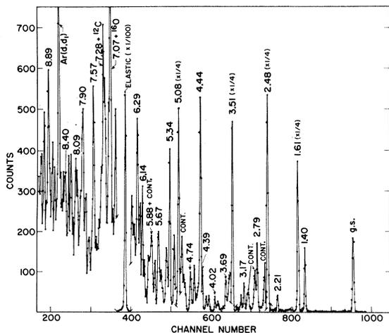
FIG. 1.  $^{36}\text{Ar}(d,p)^{37}\text{Ar}$  pulse-height spectrum, at a center-of-target deuteron energy of 9.162 MeV and lab angle of 50.0°.
