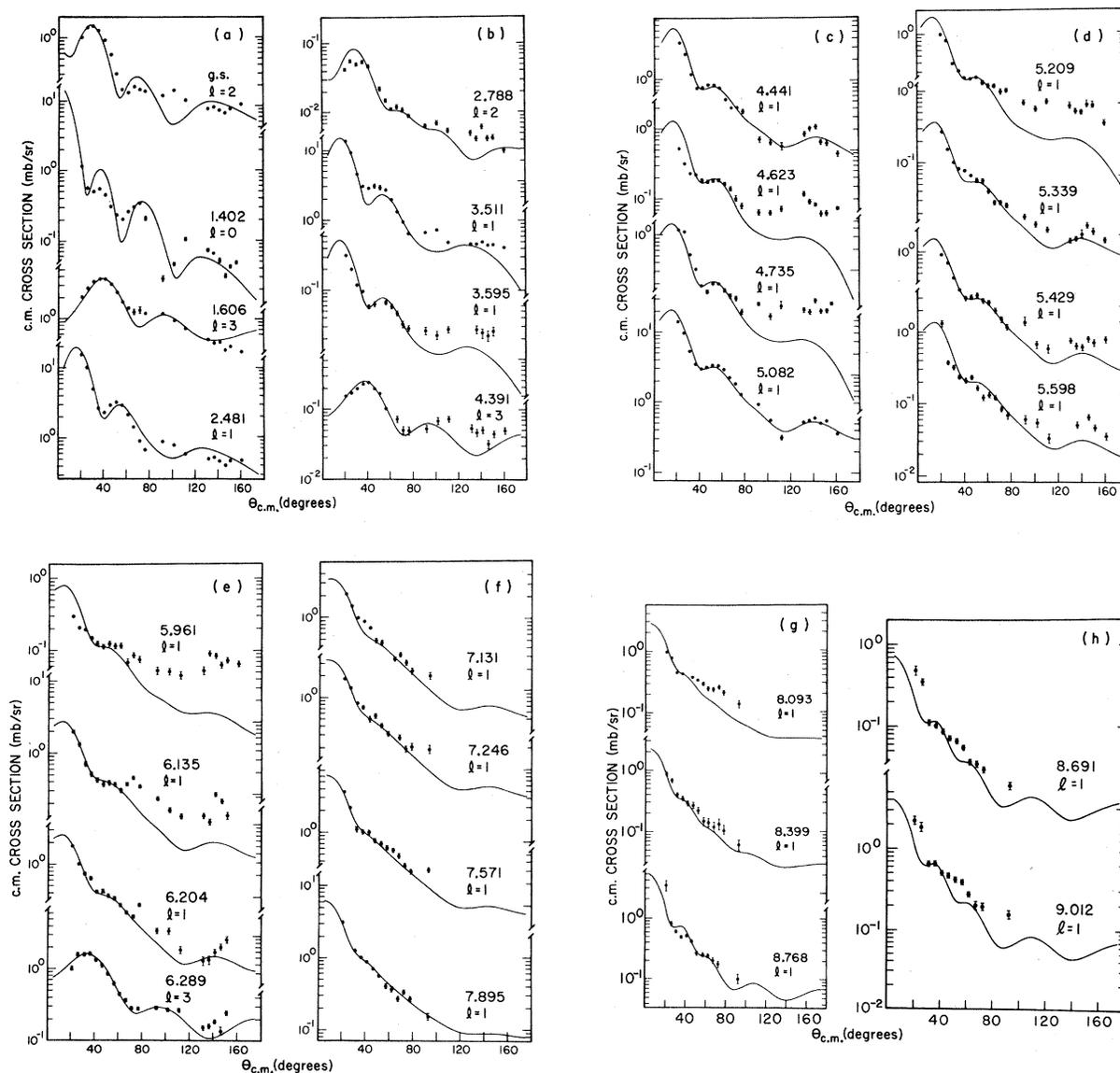
FIG. 4. DWBA fits to the  $^{36}\text{Ar}(d, p)^{37}\text{Ar}$  angular-distribution data. The  $l$  values and the excitation energies are indicated. Where error bars are not used, the size of the data point indicates the approximate statistical error in the cross sections.
