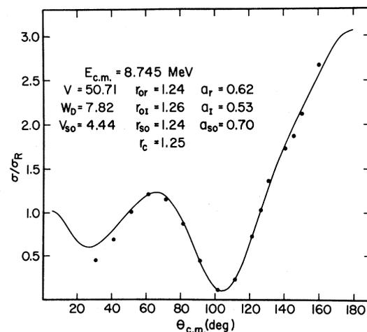
FIG. 2. Optical-model fit to the  $^{36}\text{Ar}(p,p)$  elastic scattering data. The cross section is shown as a ratio to the corresponding Rutherford cross section.
