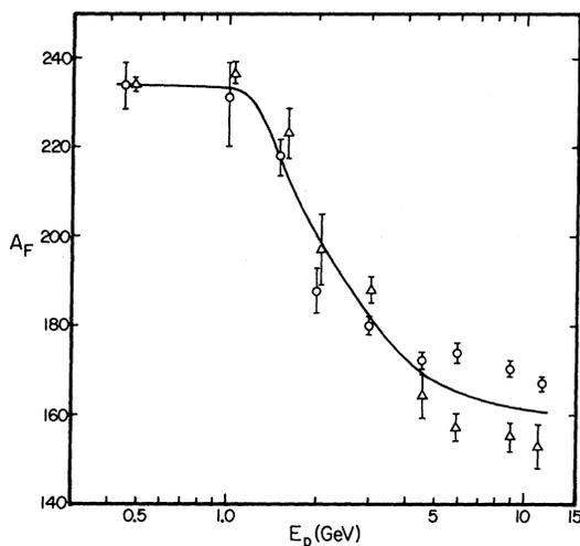
FIG. 8. Energy dependence of the mass number of the average fissioning nucleus leading to the formation of  $\text{Sr}^{83}$  ( $\Delta$ ) and  $\text{Ba}^{131}$  (o).
