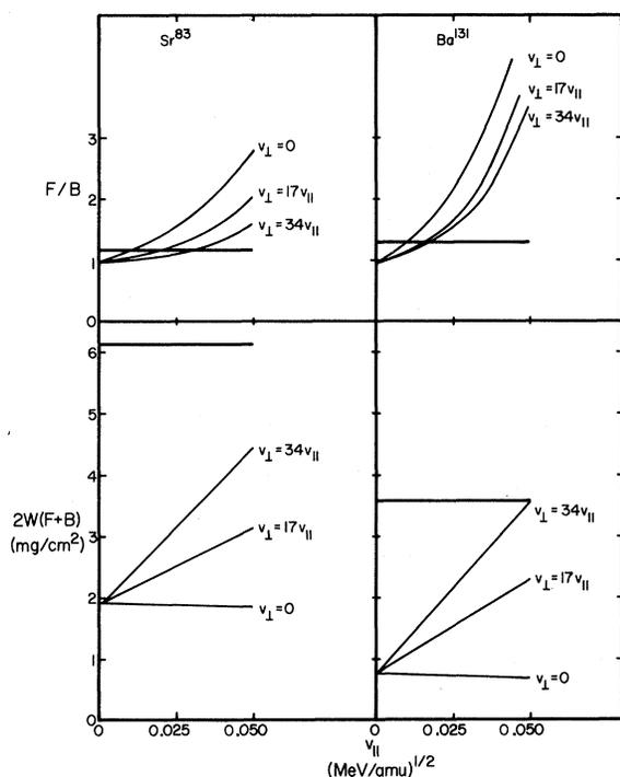
FIG. 9. Results of the spallation calculation of  $2W(F+B)$  and  $F/B$  values of products with  $A=81-85$  (left panel) and  $A=128-133$  (right panel). The calculated values are plotted as a function of  $v_{\parallel}$  for different values of  $v_{\perp}/v_{\parallel}$ . The experimental values for  $\text{Sr}^{83}$  and  $\text{Ba}^{131}$  are shown as the heavy horizontal lines.
