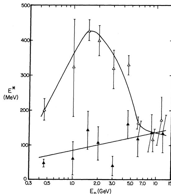
FIG. 7. Energy dependence of the average deposition energy of residual nuclei leading to  $Sr^{83}$  ( $\Delta$ ) and  $Sr^{91}$  ( $\blacktriangle$ ).
