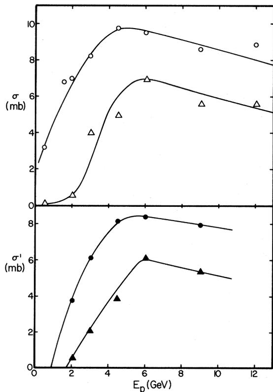
FIG. 5. Top panel - excitation functions for the formation of Ba<sup>131</sup> (o) and Sr<sup>83</sup> (Δ); bottom panel - excitation functions for the formation of Ba<sup>131</sup> (●) and Sr<sup>83</sup> (▲) by the high-energy mechanism.
