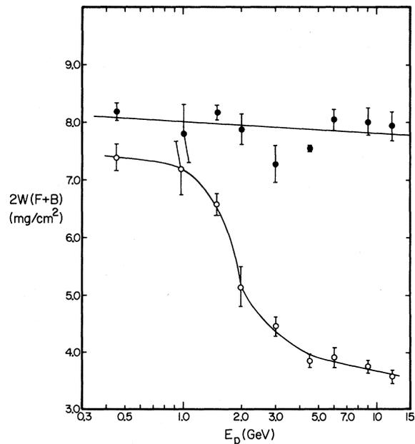
FIG. 1. Energy dependence of the experimental ranges  $[2W(F+B)]$  of  $Ba^{131}$  (o) and  $Ba^{140}$  (●).
