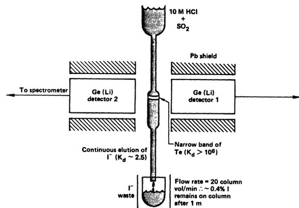
FIG. 1. Counting arrangement for samples of  $^{133}\text{Te}^m$ .
