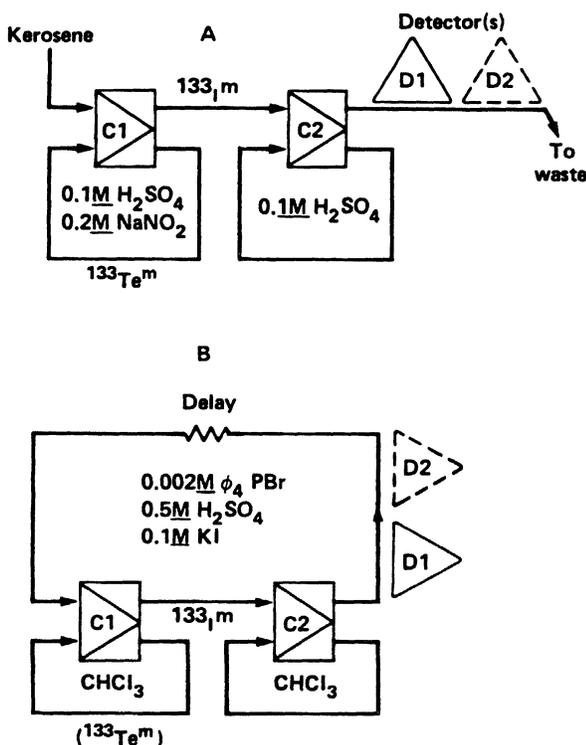
FIG. 2. SISAK configurations used to isolate 9-s  $^{133}\text{I}^m$  from  $^{133}\text{Te}$ .
