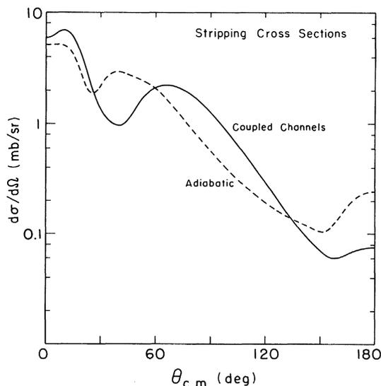
FIG. 5. Stripping cross sections for the case described in the text taken from the CC theory (Ref. 4) (solid line), and the adiabatic theory (Ref. 11) (dotted line).
