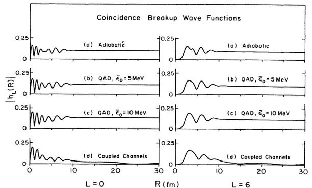
FIG. 2. Coincidence breakup functions  $|h_L(R)|$  for partial waves  $L = 0, 6$  from (a) adiabatic theory, (b) QAD with  $\bar{\epsilon}_L = (5 \text{ MeV}) \exp(-L/12)$ , (c) QAD with  $\bar{\epsilon}_L = (10 \text{ MeV}) \exp(-L/12)$ , (d) CC theory.
