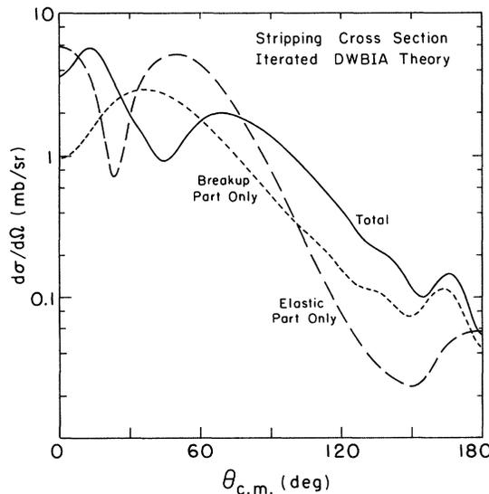
FIG. 9. Stripping cross section as in Fig. 5, computed with the DWBIA iterated theory of Eq. (2.33), with closed channels excluded by an upper cutoff at  $k = 0.72 \text{ fm}^{-1}$ . Total wave function used (solid line), only breakup wave function (dotted line), and only elastic wave function (dashed line).
