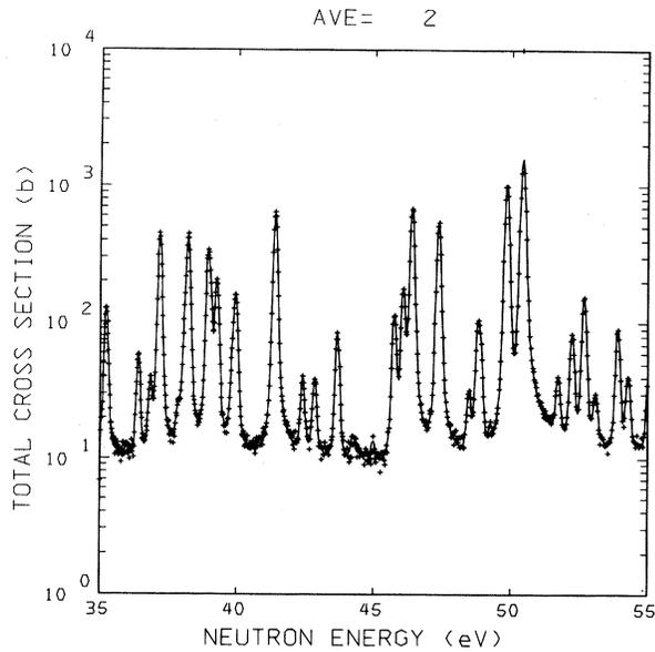
FIG. 1. Neutron total cross section of  $^{237}\text{Np}$  from 35 to 55 eV. The data have been averaged by two time-of-flight channels. The solid curve represents the one-channel  $R$ -matrix fit to the data.
