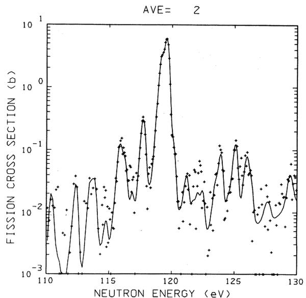
FIG. 4. Neutron fission cross section of  $^{237}\text{Np}$  from 110 to 130 eV. The data have been averaged by two time-of-flight channels. The solid curve represents the one-channel  $R$ -matrix fit to the data.
