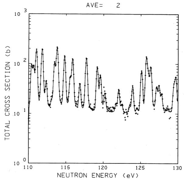
FIG. 3. Neutron total cross section of  $^{237}\text{Np}$  from 110 to 130 eV. The data have been averaged by two time-of-flight channels. The solid curve represents the one-channel  $R$ -matrix fit to the data.
