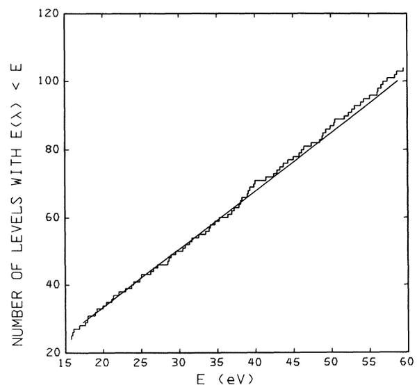
FIG. 6. Cumulative staircase plot of the number of levels  $E_\lambda$  with an energy  $< E$  vs the neutron energy for the energy region from 15 to 60 eV. The solid curve represents a linear fit to the data below 40 eV.
