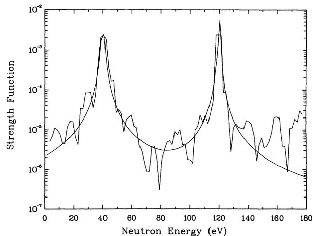
FIG. 8. Fission strength function for  $^{237}\text{Np} + n$  from 0 to 180 eV. The smooth curve is typical of the fit for either the narrow- or broad-level case.
