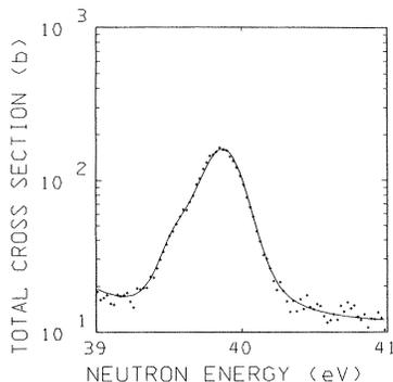
FIG. 5. Neutron total cross section of  $^{237}\text{Np}$  in the region of the 39.9-eV resonance. The 39.7-eV resonance is clearly evident on the low-energy side of the 39.9-eV resonance.
