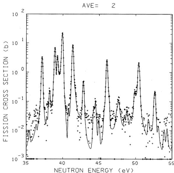
FIG. 2. Neutron fission cross section of  $^{237}\text{Np}$  from 35 to 55 eV. The data have been averaged by two time-of-flight channels. The solid curve represents the one-channel  $R$ -matrix fit to the data.
