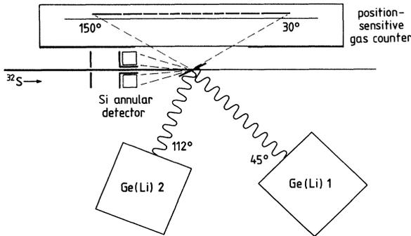
FIG. 1. Experimental setup used in the present Coulomb-excitation study.
