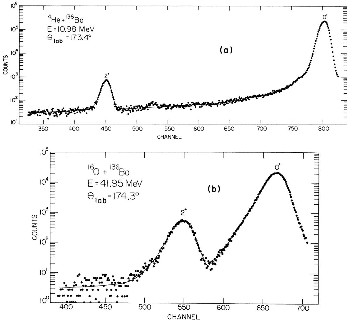
FIG. 1. Spectra of  $^4\text{He}$  ions (a) and  $^{16}\text{O}$  ions (b) back-scattered from  $^{136}\text{Ba}$ . The lines passing through the experimental points represent the fits to the spectra from which the contributions of scattering from contaminants were subtracted.
