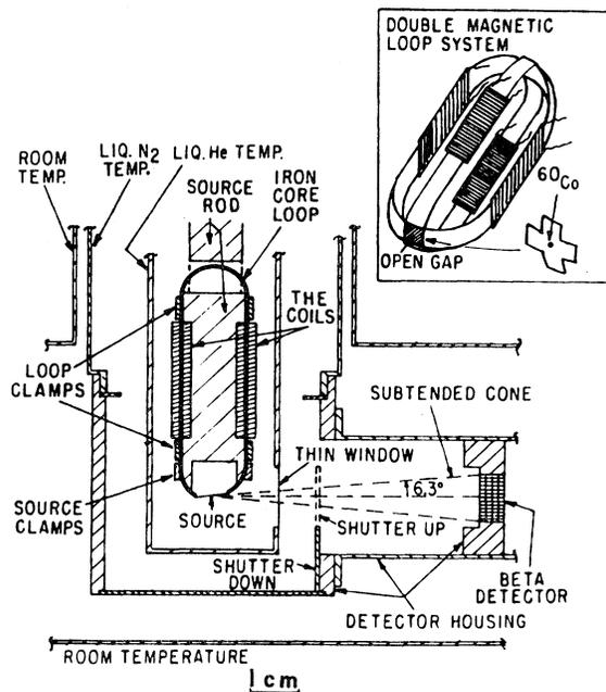
FIG. 2. Cross-sectional view of the  $^3\text{He}/^4\text{He}$  dilution refrigerator tail section used in the  $\beta$  asymmetry measurements. The permendur source foil is clamped to the double magnetic loop system in the region labeled "source."
