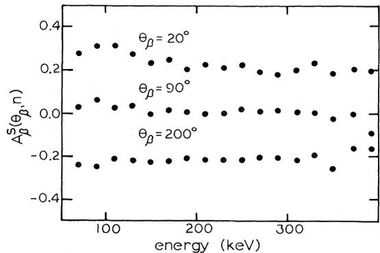
FIG. 4.  $^{58}\text{Co}$   $\beta^+$  asymmetry versus the  $\beta^+$  energy. The angles listed are those between the nuclear polarization axis and the  $\beta$  detector axis.
