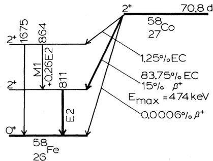
FIG. 1. Decay scheme of <sup>58</sup>Co.
