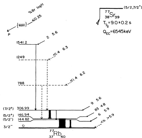
FIG. 1. Radioactive decay scheme established for  $^{77}\text{Sr}$ .
