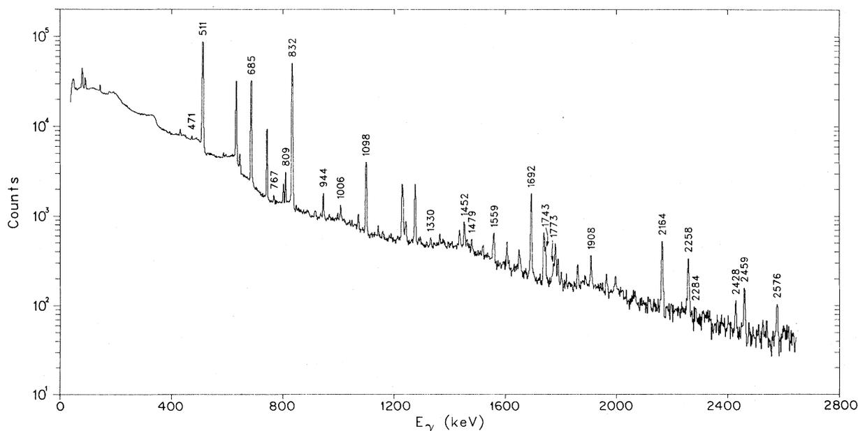
FIG. 1.  $\gamma$ -ray spectrum obtained in  $\approx 2$  h with a 40-cm<sup>3</sup> Ge(Li) detector from a metal foil containing both 1.55-min and 9.25-min  $^{96}\text{Rh}$  activities. All energies are in keV. All  $\gamma$  rays definitely ascribed to the 1.55-min  $^{96}\text{Rh}$  isomer are labeled in the figure.
