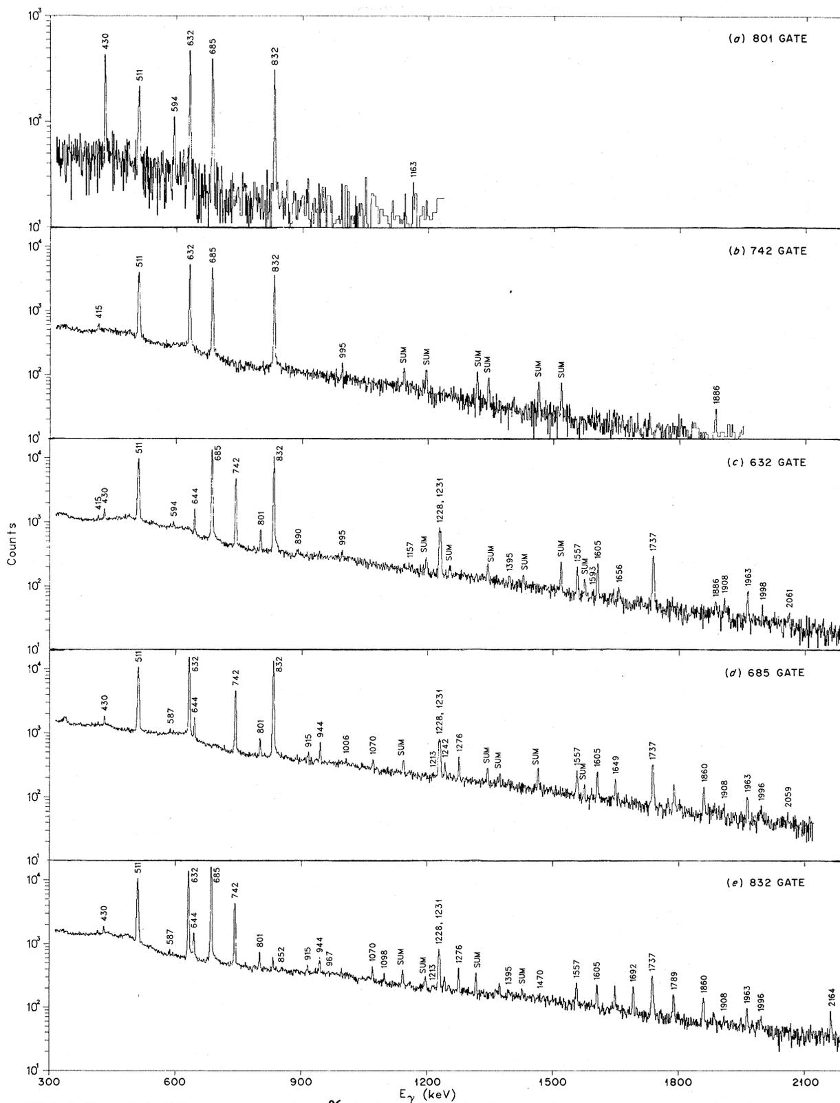
FIG. 3. Typical Ge(Li)  $\gamma$ -ray spectra from  $^{96}\text{Ru}$  observed in coincidence with various  $\gamma$  ray gates selected by a second Ge(Li) detector. All energies are in keV. Contributions to the spectra due to Compton events present within the gate have been subtracted.
