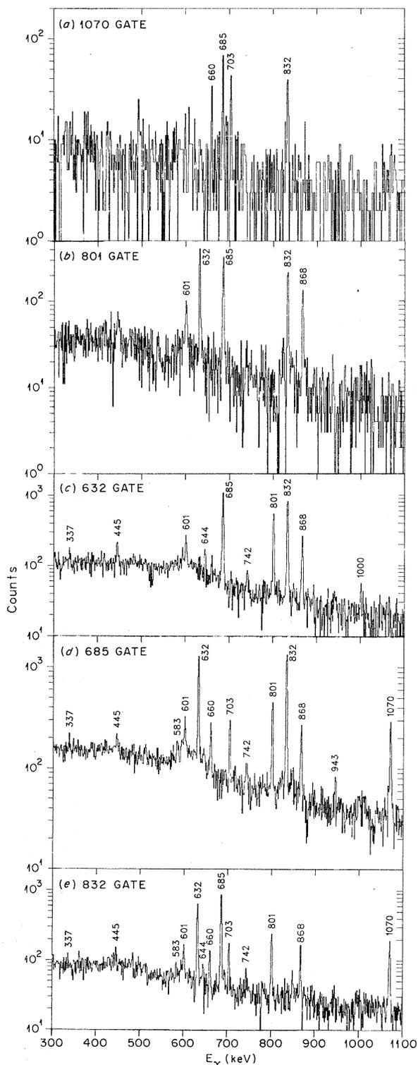
FIG. 4. Typical Ge(Li)  $\gamma$ -ray spectra from the  $^{93}\text{Nb}(^6\text{Li},3n\gamma)$  reaction observed in coincidence with various  $\gamma$  ray gates selected by a second Ge(Li) detector. All energies are in keV. Contributions to the spectra due to Compton events present within the gate have been subtracted.
