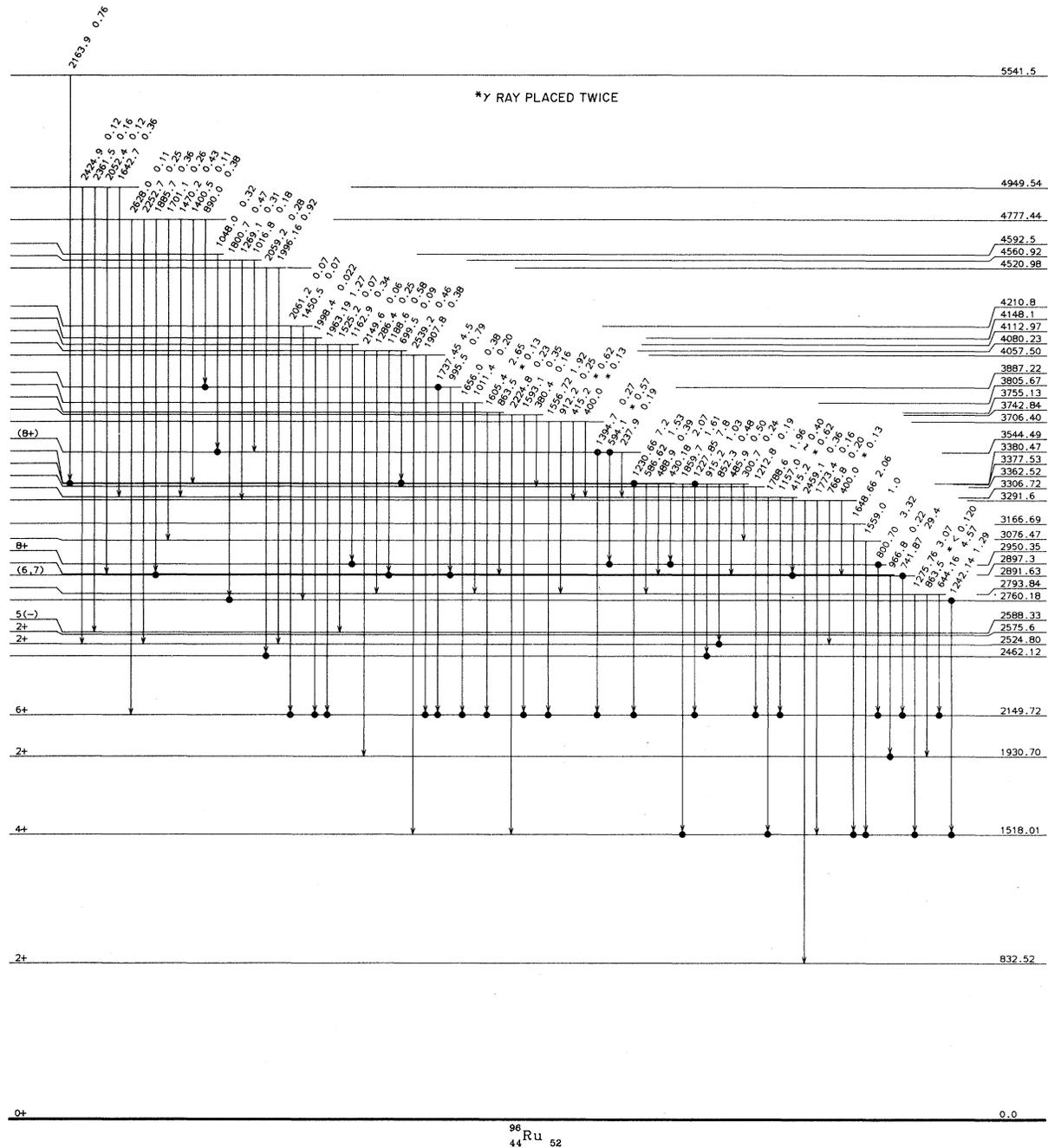
FIG. 5. Proposed decay schemes for  $^{96}\text{Rh}$  isomers. All energies are in keV. The heavy dots indicate coincidences. The numbers next to the  $\gamma$ -ray energies denote the absolute transition intensities per 100 disintegrations of the parent. In the case of the low- $J$   $^{96}\text{Rh}$  decay, the intensity of the isomeric transition (not shown) was assumed to be 60% (Ref. 5).
