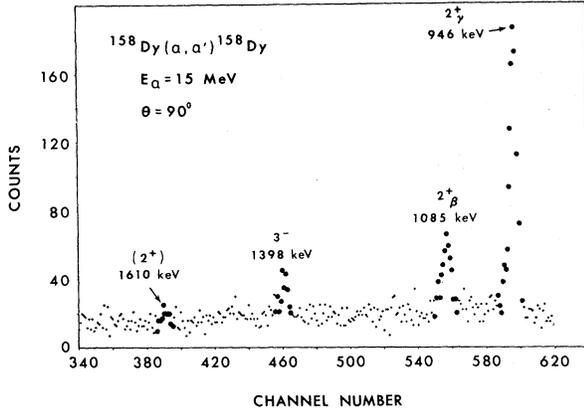
FIG. 2. Alpha particle spectrum for low-lying vibrational states in  $^{158}\text{Dy}$ . The lowest lying  $I^\pi K=2^+0$  state at 1085 keV is much more strongly excited than the 828 keV state in  $^{156}\text{Dy}$ , as seen by comparing this spectrum with the one in Fig. 1.
