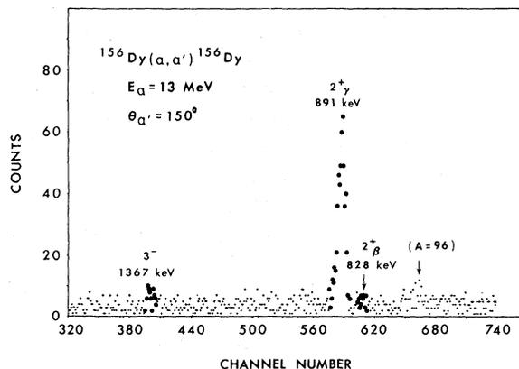
FIG. 1. Alpha particle spectrum for low-lying vibrational states in  $^{156}\text{Dy}$ . Although the 828 keV state is labeled " $\beta$ ," it is not collective.
