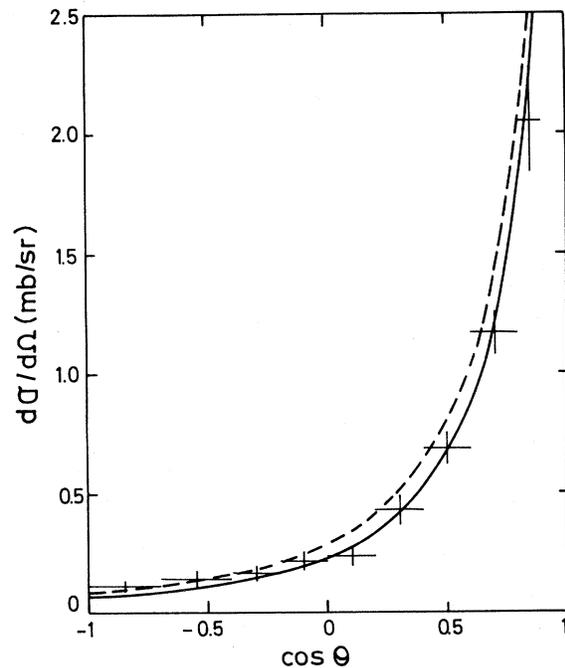
FIG. 2. Comparison of the elastic  $K^+d$  differential cross sections in the laboratory frame evaluated by means of the Faddeev equations (continuous curve) and in the single-scattering impulse-approximation (dashed curve) at 342 MeV/c  $K^+$  incident momentum. The two-body potentials used in both calculations are those mentioned in the text, with a  $I=0$   $K^+N$   $S$ -wave scattering length  $a_0 = -0.015$  fm. The experimental points are the same as in Fig. 1.
