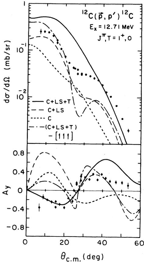
FIG. 11. DWIA calculations for the 12.71-MeV state of  $^{12}\text{C}$ . See also the caption for Fig. 5.
