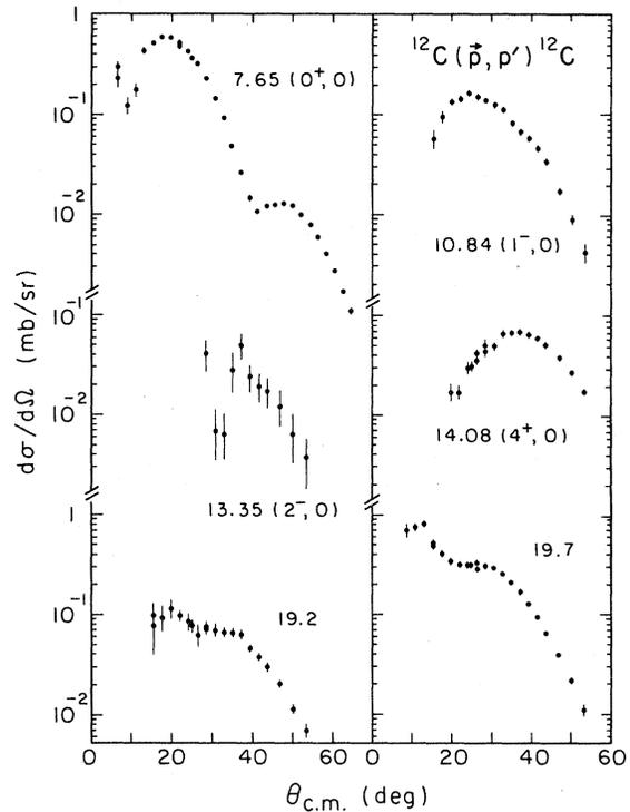
FIG. 2. Differential cross sections for excited states of  $^{12}\text{C}$ . The excitation energies are given in units of MeV and the  $J^\pi, T$  values are listed where known.
