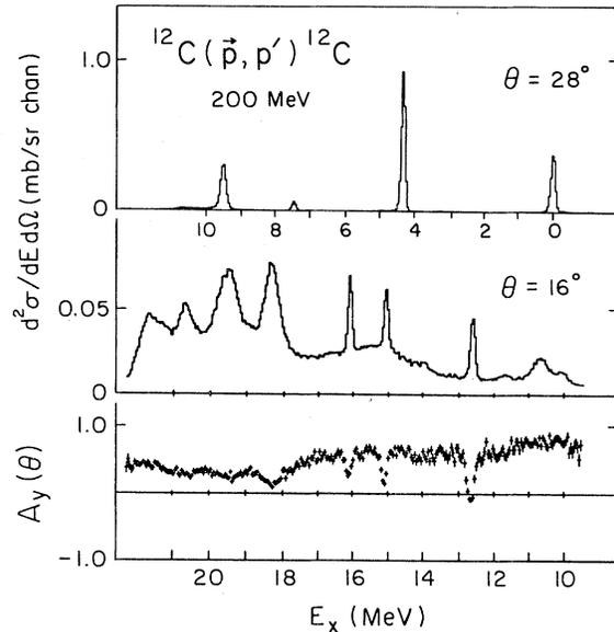
FIG. 1. Sample spectra of the equivalent unpolarized cross sections for the  $^{12}\text{C}(\vec{p}, p')^{12}\text{C}$  reaction at 200 MeV plotted against excitation energy. The analyzing powers for the high-excitation region are shown in the bottom segment.
