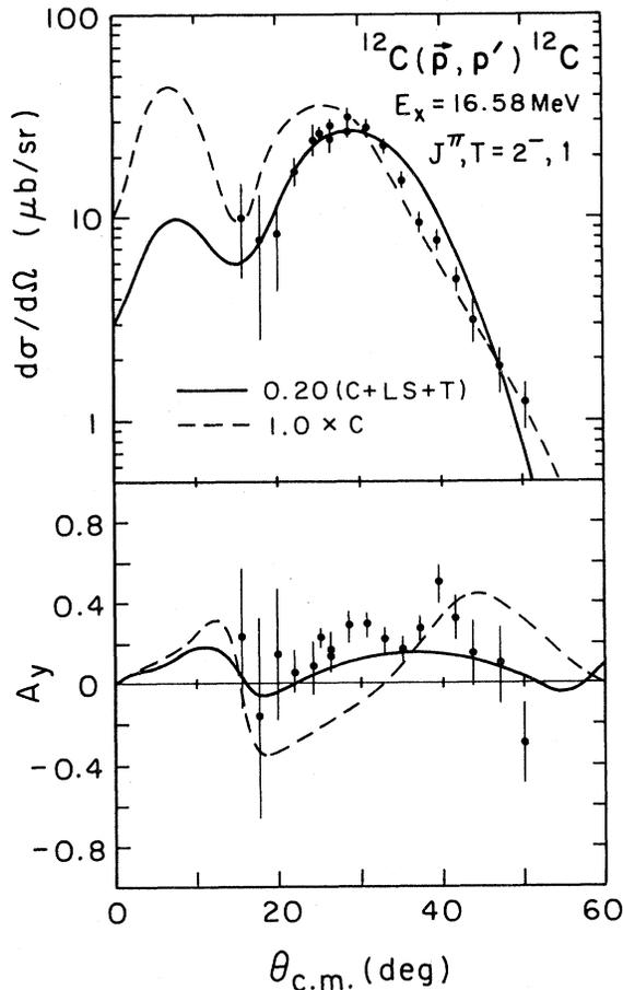
FIG. 6. DWIA calculations for the 16.58-MeV state of  $^{12}\text{C}$ . See also the caption for Fig. 5. The theoretical cross sections shown by the solid curve have been divided by 5.
