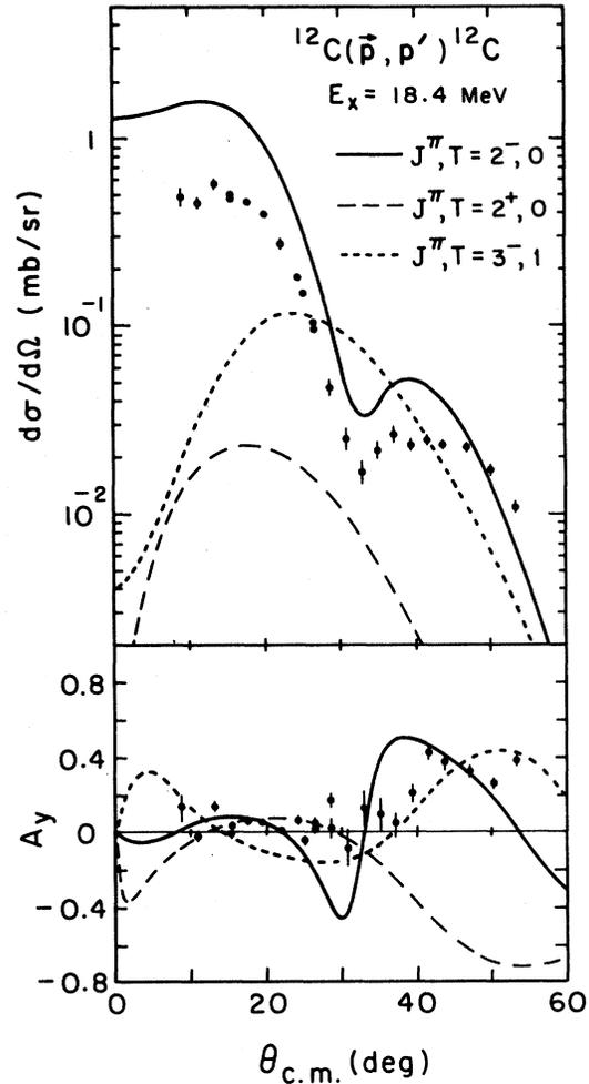
FIG. 13. DWIA calculations for the 18.4-MeV state of  $^{12}\text{C}$  with three choices for the  $J^\pi$ ,  $T$  of the state.
